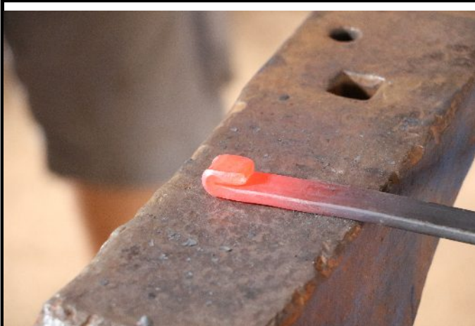
Step 3: Bend the bar back onto itself. This part will form the nose and mouth.
