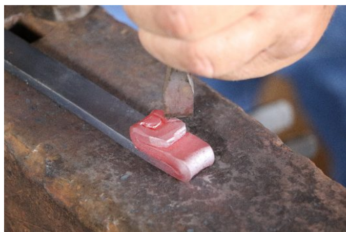
Step 8: Take the straight chisel and make whiskers along each side of the mouth. If you prefer, you can also use the center punch to put dimples in on each side for a different type of whisker look. But I prefer the straight lines.
