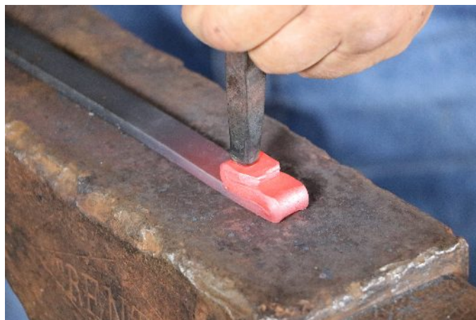
Step 7: Take the mouth punch and make an upside down "U" shape for the mouth.
