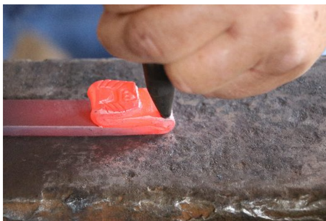
Step 12: Form the ears with the small Ball Punch. Go into the material at a slight angle to push them up and out from the head.
