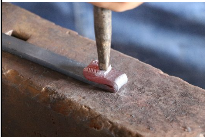
Step 9: Punch in the triangular nose shape.
