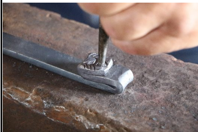
Step 10: Use the center punch to make two nostrils.
