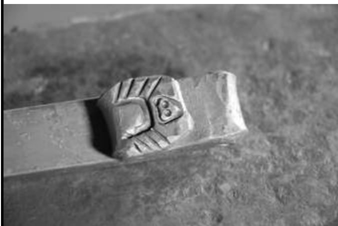
Step 11: Progress so far. If anything gets out of line, go ahead and tidy it up with light hammer blows. Be careful not to damage any of the facial features you have forged in so far.
