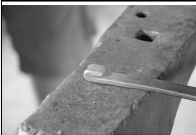
Step 3: Bend the bar back onto itself. This part will form the nose and mouth.
