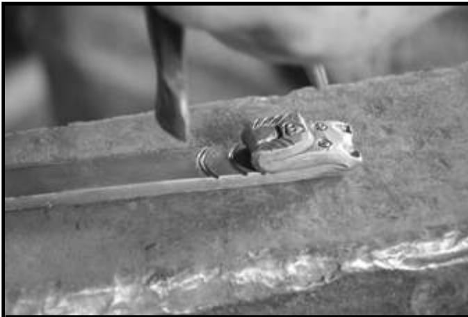
Step 15: With the curved chisel, make a pair of lines to define the collar. (I am showing double lines here because the chisel skipped but a pair of single lines is just fine.)
