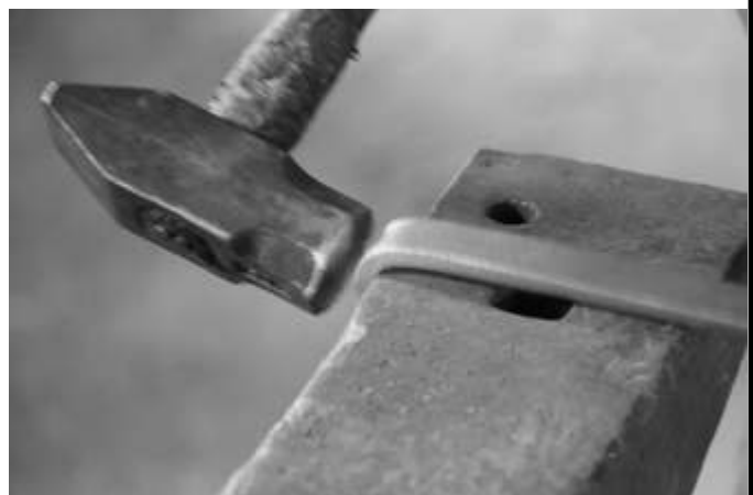
Step 2: Bend the end of the bar on the edge of the anvil. I bend about the same length as the bar is wide.
