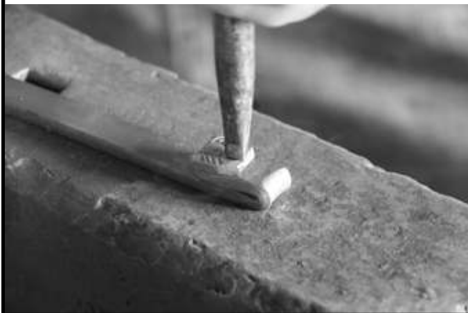
Step 9: Punch in the triangular nose shape.
