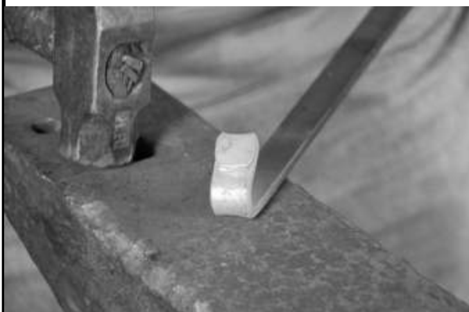
Step 5: Bend the bar back onto itself as with the first bend. Leave about half as much bar showing on the second bend as the original bend. This part will form the eyes and ears. Adjust the proportions by hammering the end of the original bend as you make the second bend if necessary.
