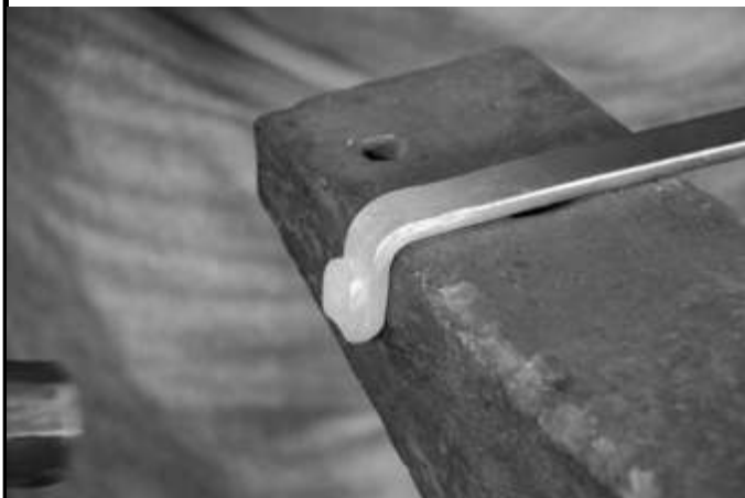
Step 4: Bend the bar on the edge of the anvil again, this time with the original fold to the outside.
