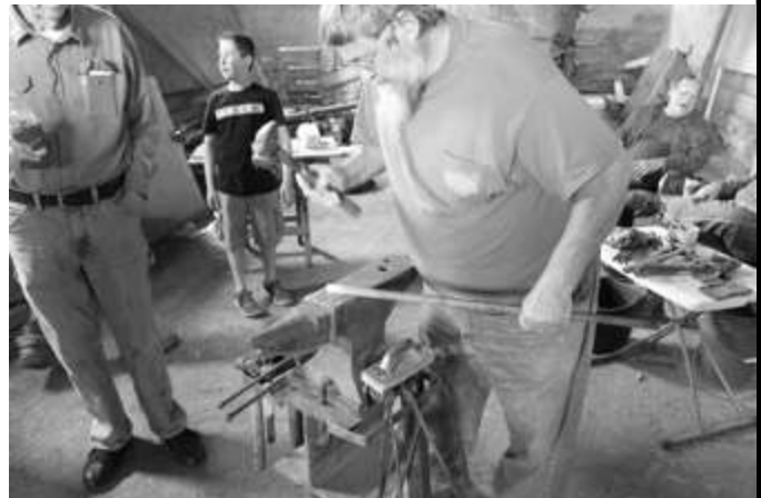
Step 1: I start by breaking the corners on the end of the bar
