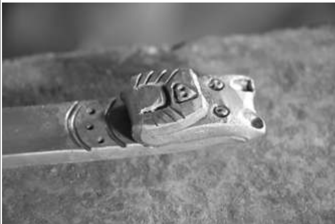
Step 16: With the center punch, place some dots on the center of the collar for a more detailed look. Congratulations - his completes the dog head!
