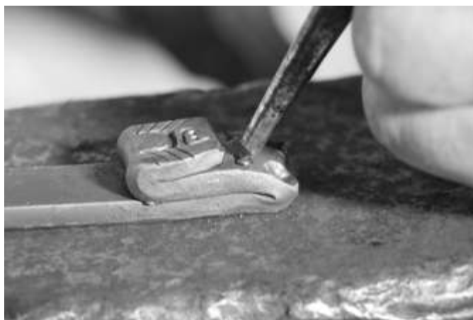
Step 14: Use the Center Punch to make pupils in each eye. Be careful to center them unless you want to create some kind of expression (rolling eyes, etc.)
