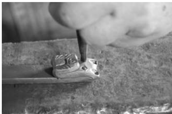
Step 13: Use the eye punch to locate the outer shape of both eyes between the nose and the ears.
