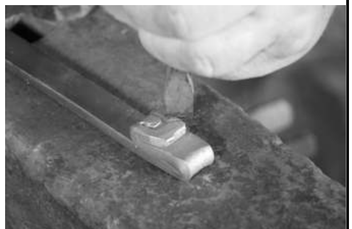
Step 8: Take the straight chisel and make whiskers along each side of the mouth. If you prefer, you can also use the center punch to put dimples in on each side for a different type of whisker look. But I prefer the straight lines.
