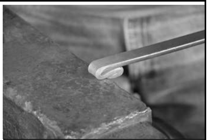
Step 6: Turn the bar over and tighten the bend. Clean up and Square up the edges.
