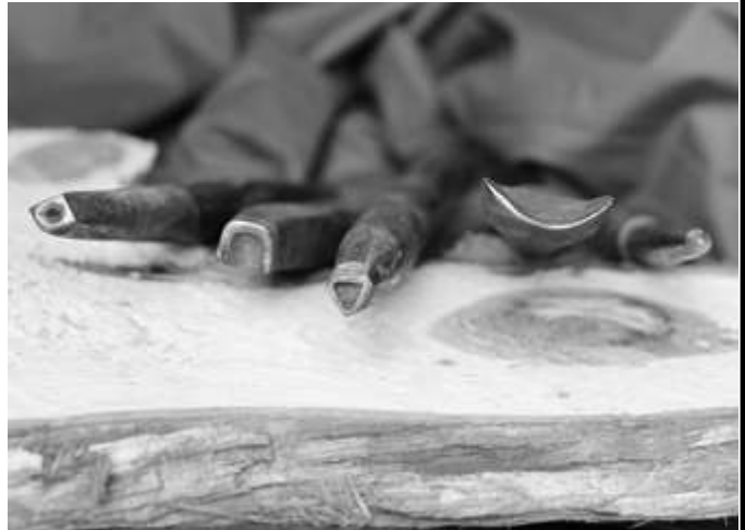
The Punches: Eye, Mouth, Nose, Collar, and Center Punch. You will also need a small Ball Punch (not shown) for the ears and a Straight Chisel for whiskers.
