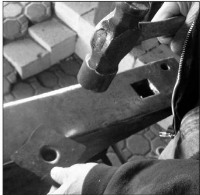
Draw out brim with rounding hammer.
