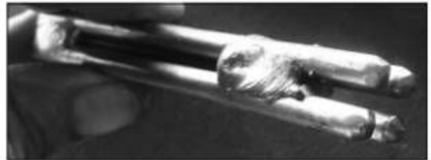
4-dimple punch for locating dimples when making a Tom Mix-style hat.
