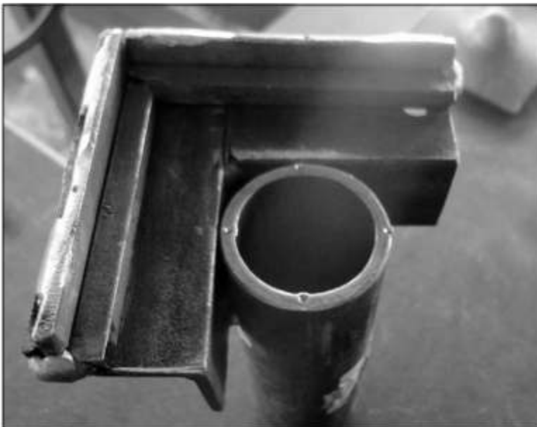
Initial Female Tool with welded-in corner reference.
