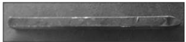
Diamond-end punch for making corrections.
