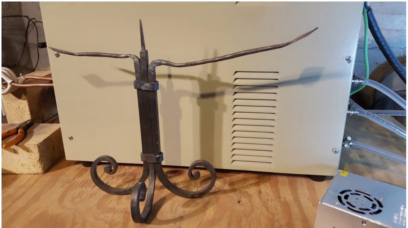
Bill Epps-style candle stand from \frac{3}{8} " square stock (still needs pan and adjustments)
