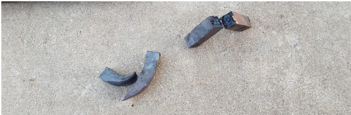
Welds tested to failure
