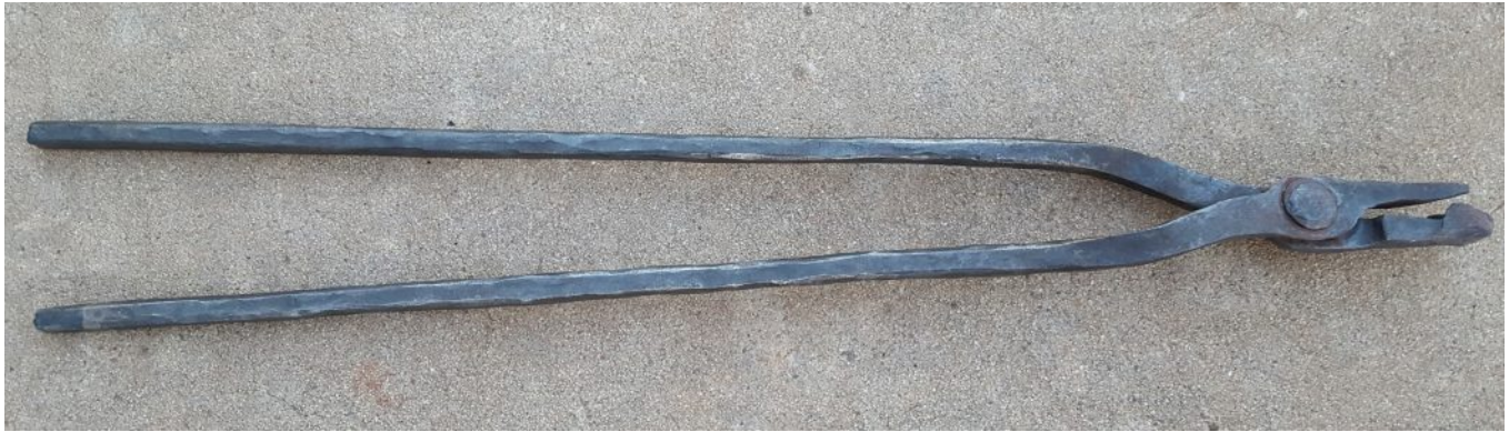
Box jaw tongs from \frac{5}{8} " sucker rod.
