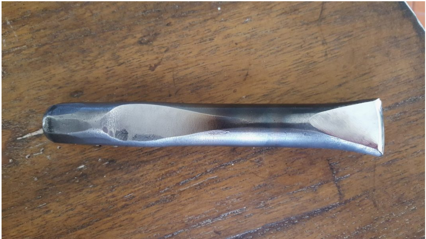
3/8" diameter fuller for chasing made from 3/4" W1 tool steel
