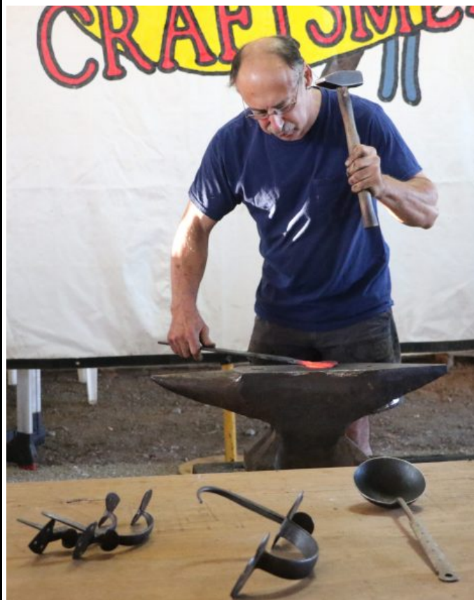
Peter's last demo was a scrolled shelf bracket showing how to correctly measure the required material and punched hole locations to get a correct fit when working
