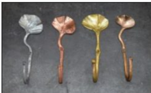
Figure 2 "J" hook in aluminum, copper, naval brass and silicon bronze
