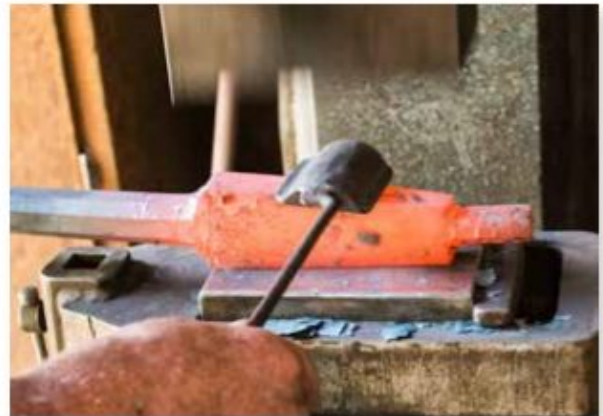
Figure 11. The auxiliary die allows Terry to refine the drift's surface.
