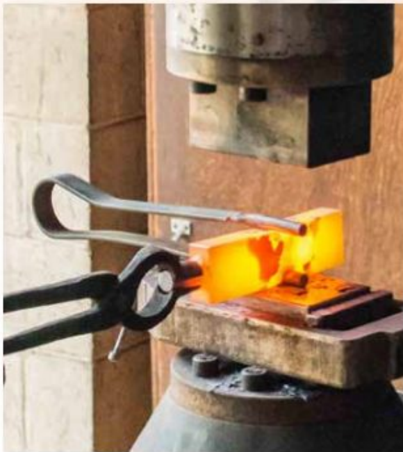
Figure 3. Using a spring fuller with a power hammer to mark off where the handle begins, at roughly midway on the bar.
