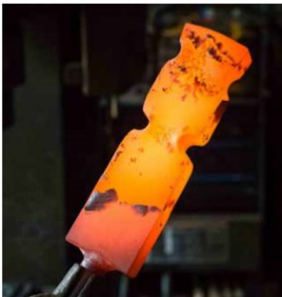
Figure 4. The spring fuller is also used to indent the steel near the end of the developing handle. Indenting at this point prevents a “bird’s mouth” from forming on the handle’s end as the bar is reduced in thickness.
