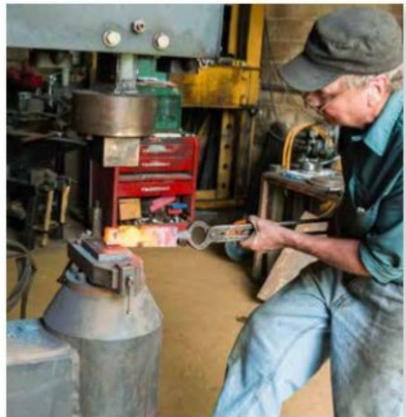
Figure 5. Terry uses the power hammer to quickly thin the bar for the handle.
