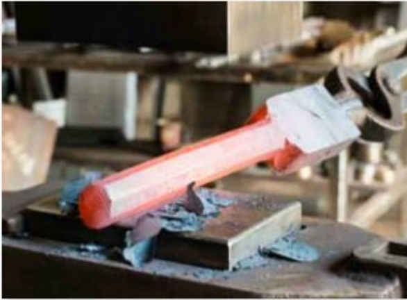
Figure 7. The handle is next forged to an octagon cross-section.
