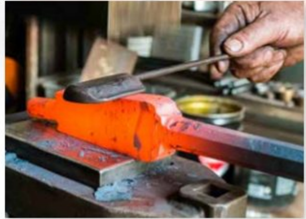
Figure 10. Using a hand-held auxiliary die with the power hammer.
