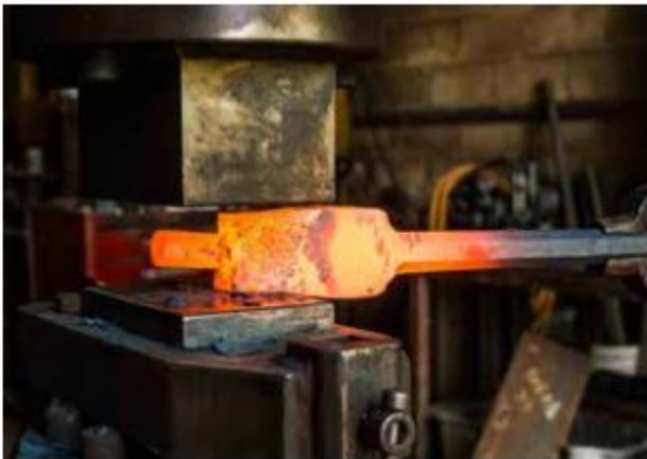
Figure 8. With the handle finished, Terry begins to forge the tapers.
