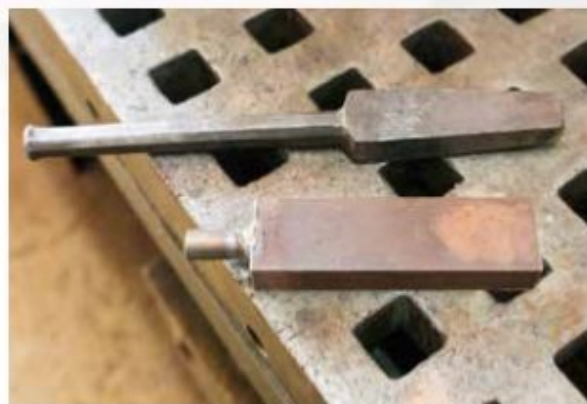
Figure 1. A finished drift and a piece of flat bar stock for making another. Note that the bar stock has a short piece of 1 inch round stock welded on to make it easier to handle the flat bar during forging. The extension can be cut off when no longer needed.
