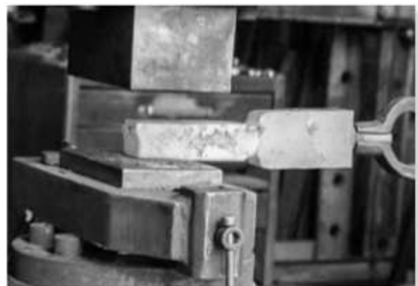
Figure 6. The handle is first forged to a square cross-section.
