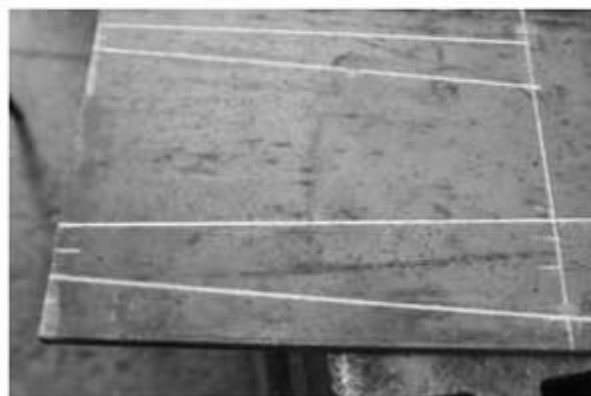
Figure 2. Terry uses chalk to sketch the tapers for the wide and narrow sides of the drift on a scrap sheet of steel.
