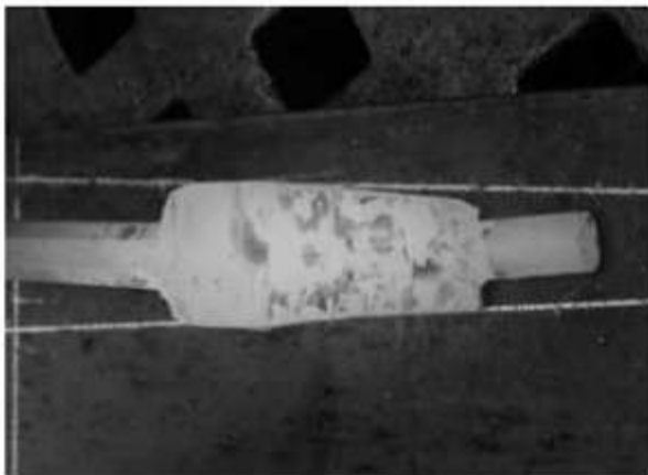
Figure 9. During forging, the developing taper is regularly compared to the template.
