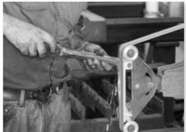
Figure 12. Terry does a final touch-up of the drift on a belt grinder.
