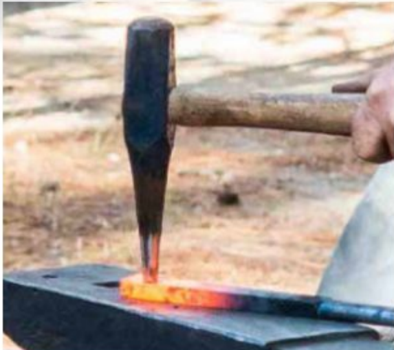
Figure 3. Punching the hole at the upper end of the pin.
