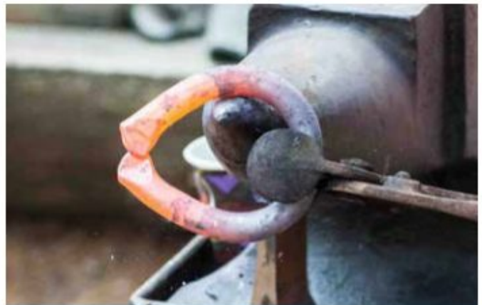
Figure 11. The centre ring ready for forge welding. Note the scarfed ends.
