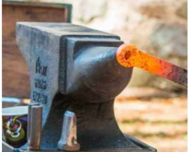
Figure 4. Refining the hole on the horn of an anvil.
