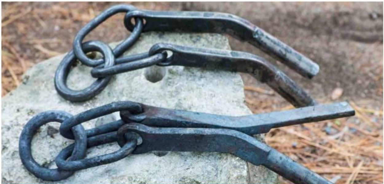
Figure 1. A pair of lewis rings. Note the hole drilled in the rock below the upper lewis ring.
