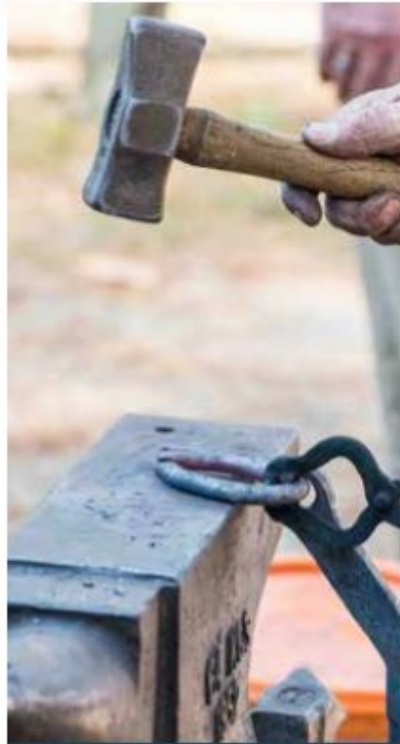
Figure 8. The chain link is attached to the pin just prior to welding.
