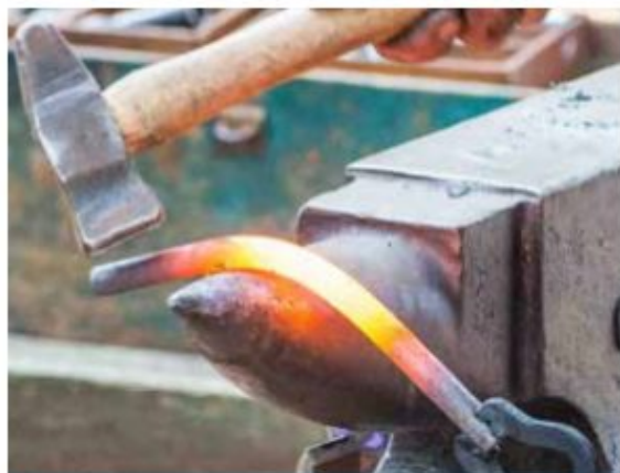
Figure 10. Beginning to form the centre ring.
