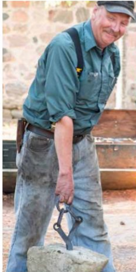
Figure 15. Terry demonstrating a lewis ring in action.
