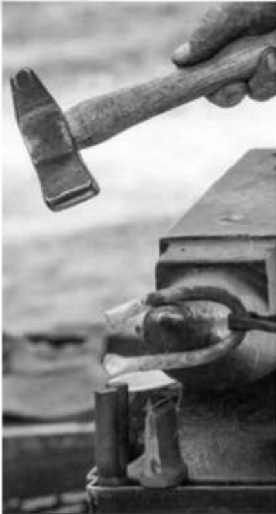
Figure 7. Forming the chain link which will attach to the end of a pin.
