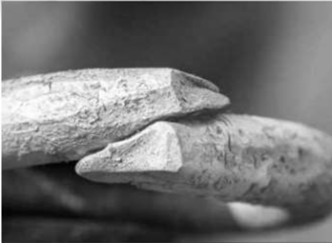
Figure 12. Close-up of the scarfed ends ready to weld.
