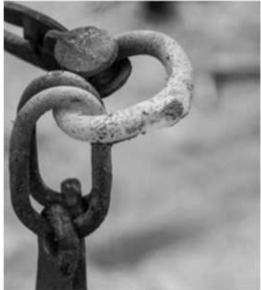
Figure 13. The centre ring after forge welding. Part of the challenge in welding the centre ring, is that you have to contend with the weight of the attached pins.
