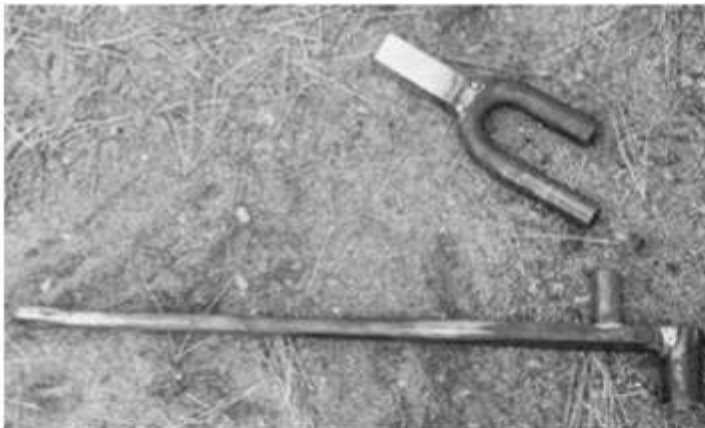
Figure 5. The jig Terry made to aid in bending the pins. The cut-off portion of the "U" provides clearance for the bending bar.
