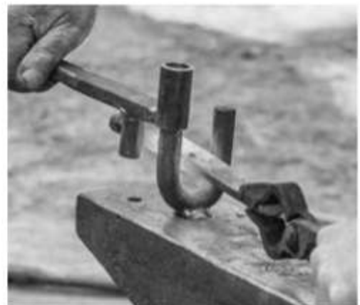
Figure 6. The bending jig in action. The pin is bent to a 30 degree angle.
