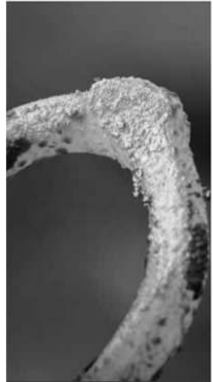
Figure 9. Detail of the chain link after initial forge welding.
