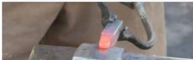
The top of the reign and piece that will form the jaw, both being scarfed to prepare for forge welding.
