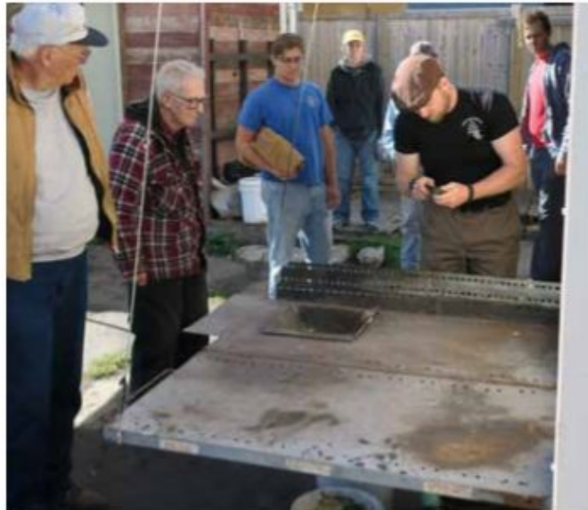
Sean's floating, legless forge that hangs from the building for easy disassembly.
