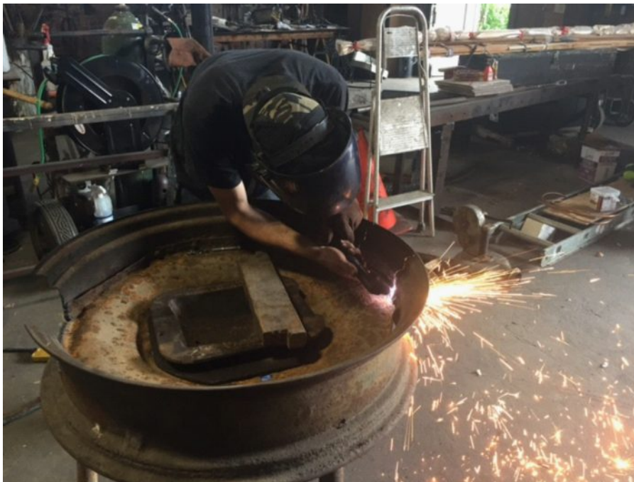
Here Daniel is cutting what I call the "pass-through" openings in the sides of the forge.
