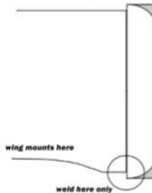
form cowl from a thick washer or some 1/8" cut to shape. Weld to fuselage at very bottom and then grind or file to contour.
