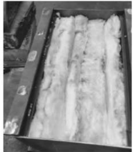
Koa wool in the lower section of the forge body
