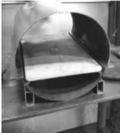
Top and bottom halves of forge shell
