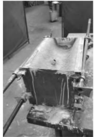
Cast refractory for top of forge Note the cast in tube for the burner insertion after the cast dries
