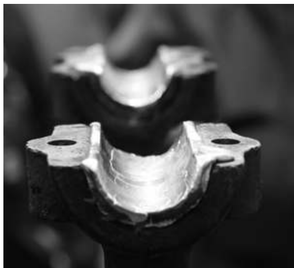
Freshly poured lower babbit bearings prior to cleanup.
