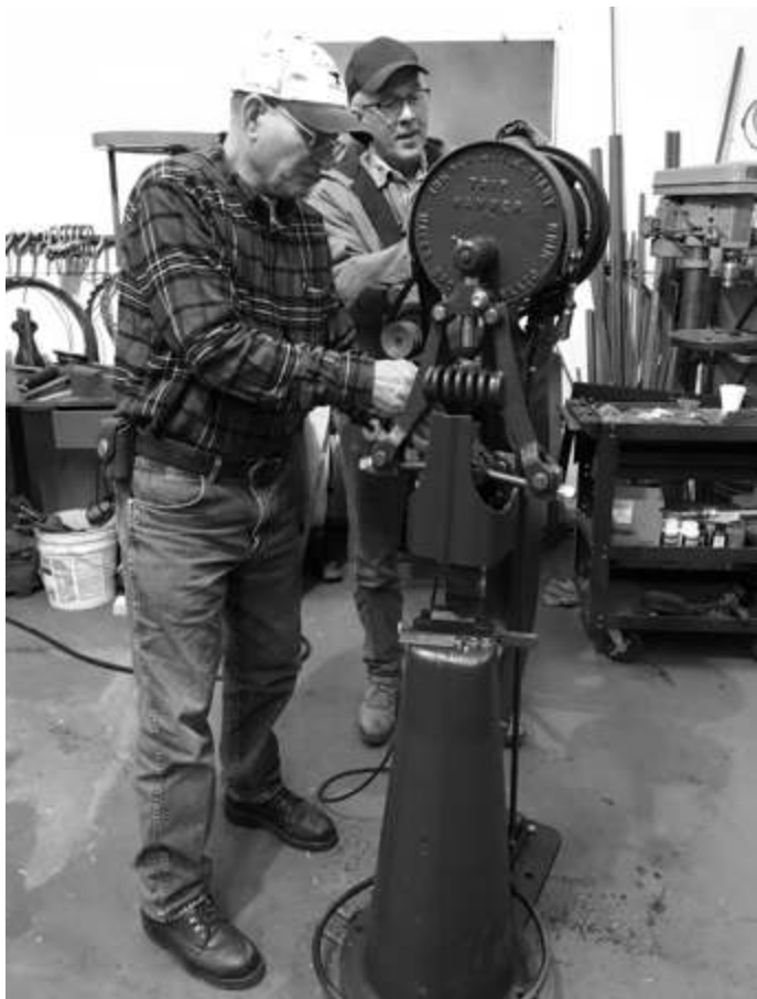
Jim Carothers and Tom Nelson making some final adjustments to the newly rebuilt hammer and installing an aftermarket brake. After new bearings and adjustments, the hammer ran silky smooth and, with the brake, was capable of making controlled single hits. And the new paint job was icing on the cake.
