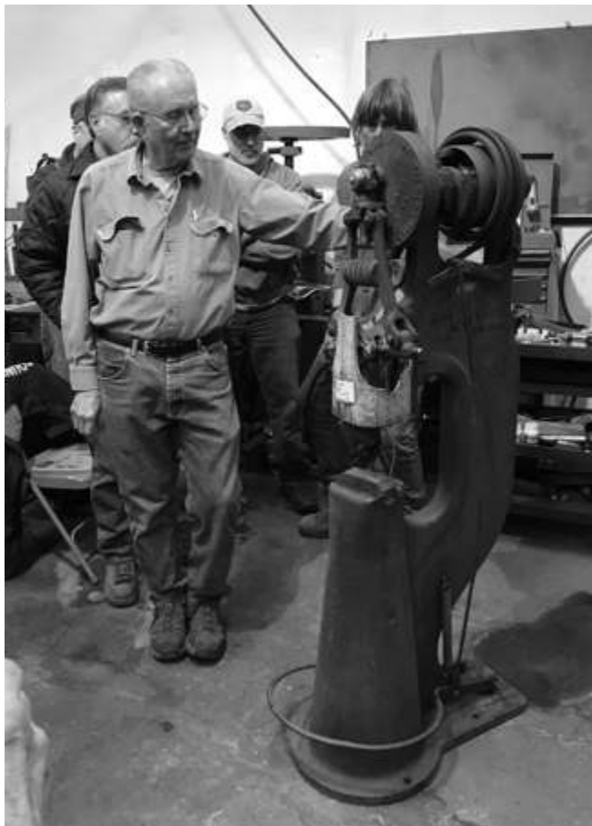
Sid Suedmeier showing the “Lazarus” hammer to the class before starting the rebuild. At this point, Sid had already done a lot of pre-cleaning. Although the hammer had numerous problems that needed to be addressed, it looked surprisingly good given its history burial and discovery by bulldozer.
