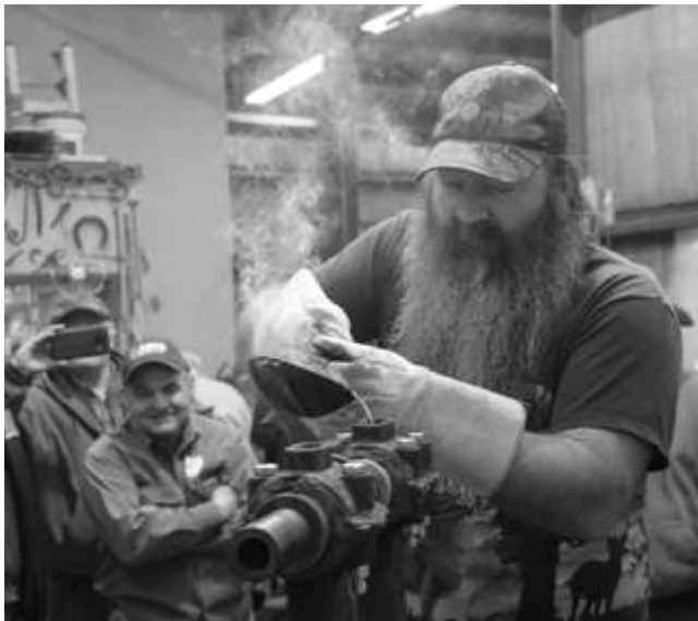
Pouring babbitt for a new upper bearing
