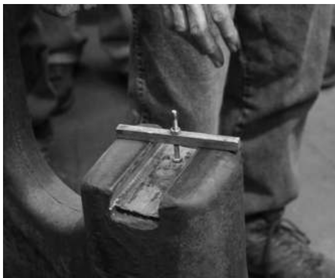
Sid demonstrating a simple jig for truing up the lower die dovetail - a common issue when rebuilding these older machines.
