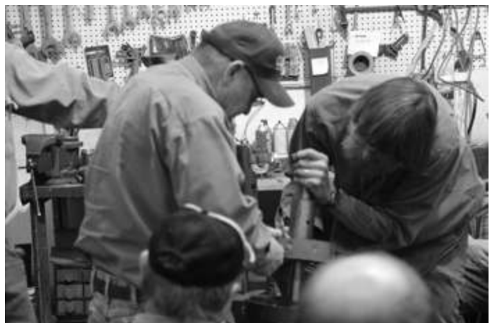
Sid demonstrating installation of new clutch lining with countersunk soft rivets
