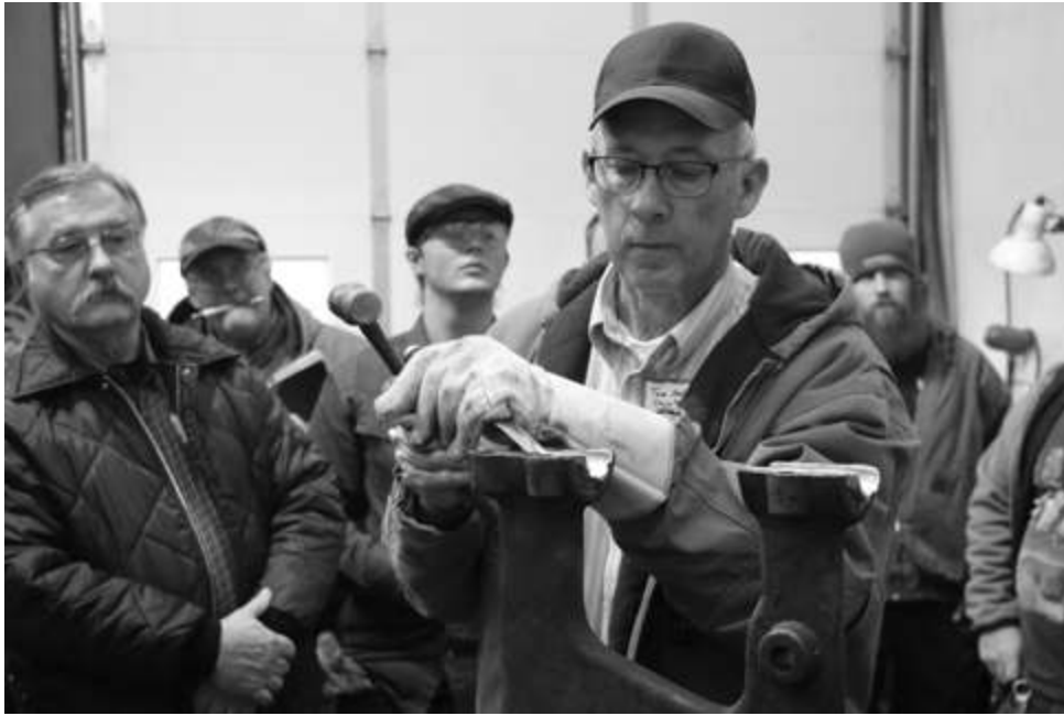
Tom Nelson cleaning up the babbitt on a newly poured lower bearing
