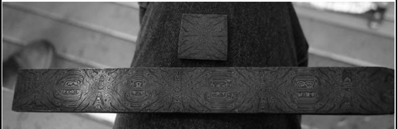
One of the Pep Gomez Mosaic Pattern Billets (End Cut and Accordion Unfold)
