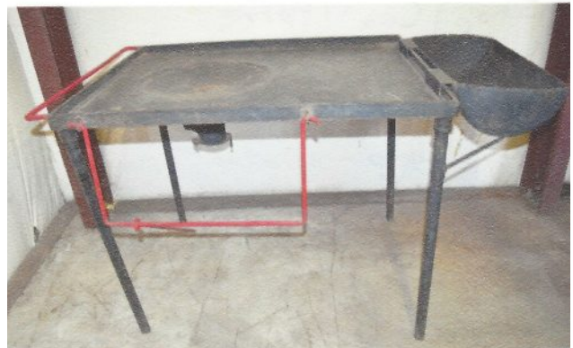
Shop Forge: 32" wide x 40" long. Tong rack, ash dump, steady rest, water trough, hood with 10" stovepipe outlet.
