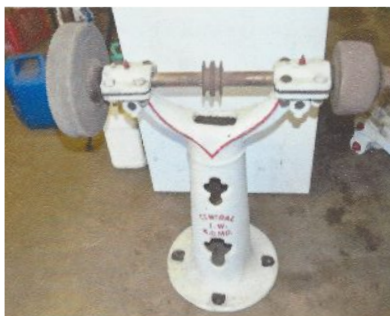
Factory Shop Pedestal Grinder: 1 1/2" arbor, Grinding Stones, no motor but has mounting bracket.
