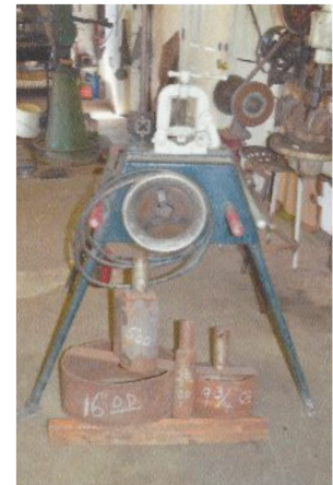
Oster Power Threader-Pipe Vice: Jigs for making rings or bands, 1-2 3/4" O.D., 1-5" O.D., 1-9 3/4" O.D., 1-10" O.D., 1-16" O.D., 1-20" O.D., Will twist 5/8" square solid bar cold.
