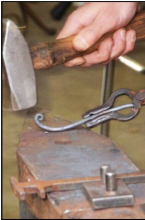
Long taper to start scroll, note open center
