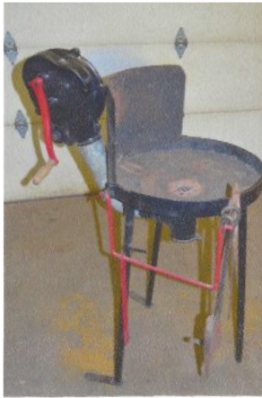
Rivet Forge (portable): 8" Champion hand-crank blower. Has wind break, tong rack, steady rest and ash dump.
