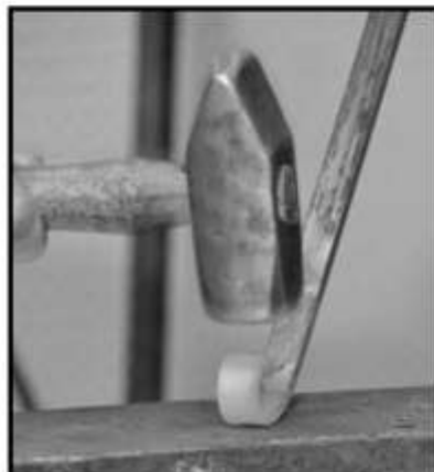
Forge small scroll end on trivet bar first
