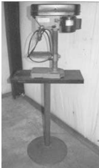
Clark Drill Press w/Stand: Ajustable chuck 0" to 1/2" capacity. Adjustable Table.
