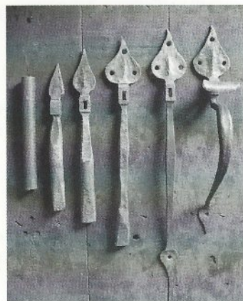
Image #2: A basic progression of a Suffolk latch from start to finish (left to right).
