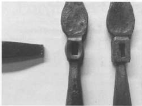
Image #6: Shows the slot punch (left), first punch (middle), and the swelling knocked in (right).
