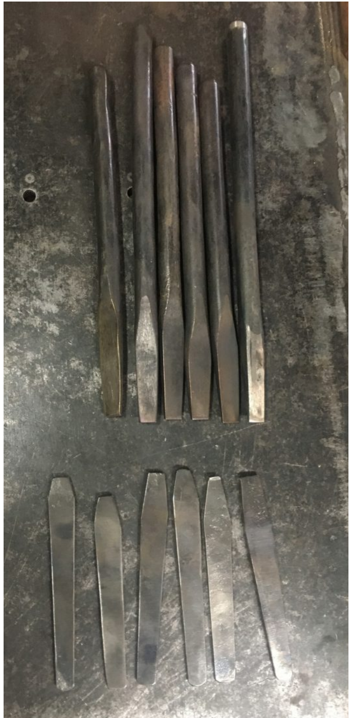
Slot Punches and Drifts by Rory Kirk (with Assistance from Don Garner) to be Used For Making Suffolk Latches
