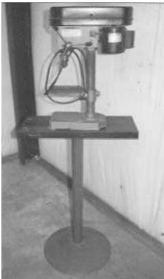
Clark Drill Press w/Stand: Adjustable chuck 0" to 1/2" capacity. Adjustable Table.
