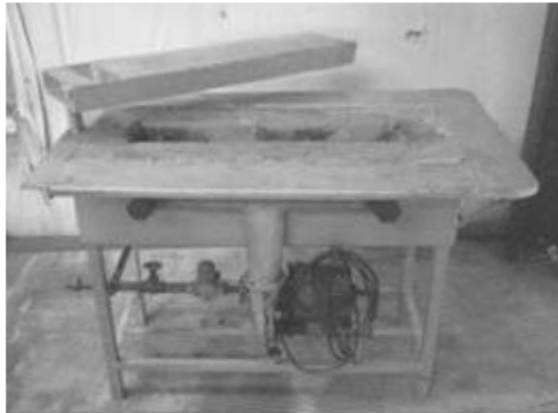
Large Johnson Gas Forge: Natural or L.P., Has 2, 3 or 4 fire burners. Fire box 12" x 30", Has L.P. Regulator and Connections, (New Fire Cement)
