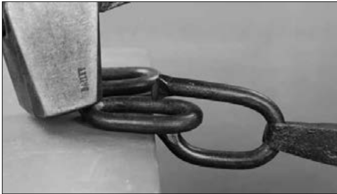
After turning one end in, pick up the other two links with the turned end down.
