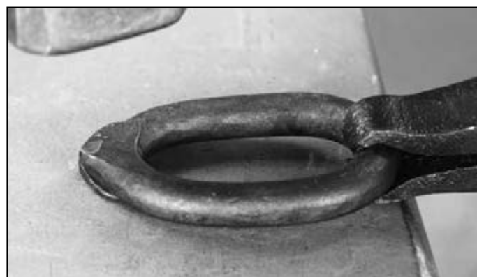
Weld on the flat face of the anvil first
