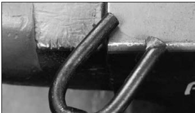
Turn the bar over and scarf the other end
