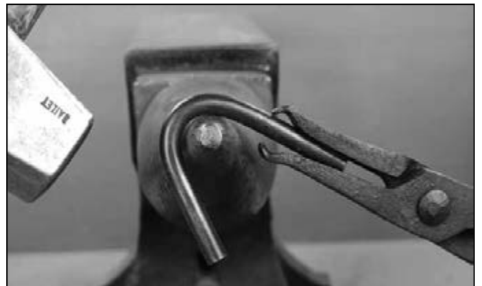
Get as far as you can working from the top, then turn the link over
