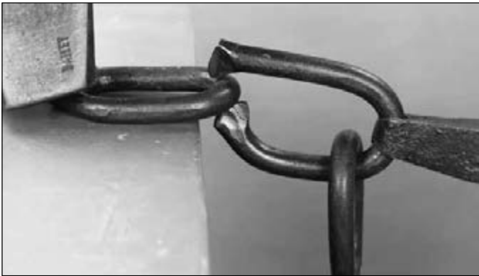
Keeping the links on the turned side will be an advantage in the next step
