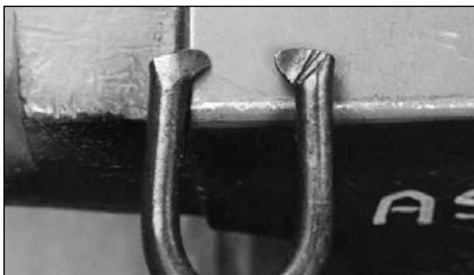
Note that the original scarf is step side up
