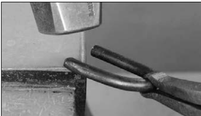
Hold your hammer at a slight angle to the anvil face
