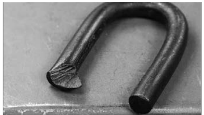
A chain-step-scarf on one end of the bar
