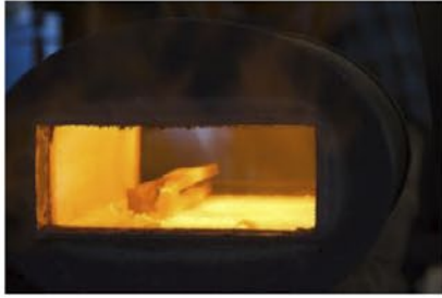
The bar partially split in the forge.
