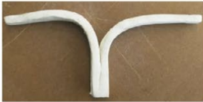
Once the splitting is done, open the chisel cuts 180 degrees at forging temperature. Drive the split on to the hardy hot cut to start spreading the split.
