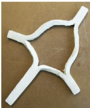
Open the corners of the splits and begin rounding over a cone or the anvil horn.
