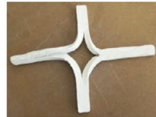
Finish opening the splits by flattening on the anvil.
