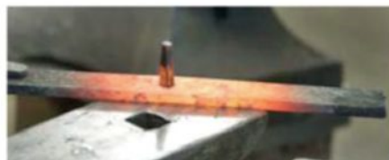
Drifting the square hole to size.
