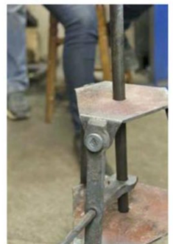
Setting the tenon in the square hole.
