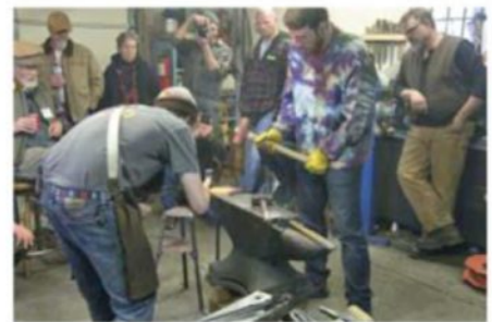
Setting the tenon in the square hole.
