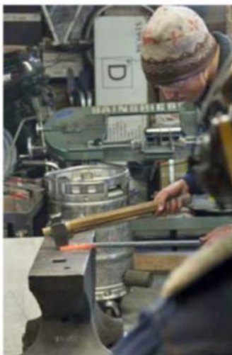
Fullering the feet before bending.
