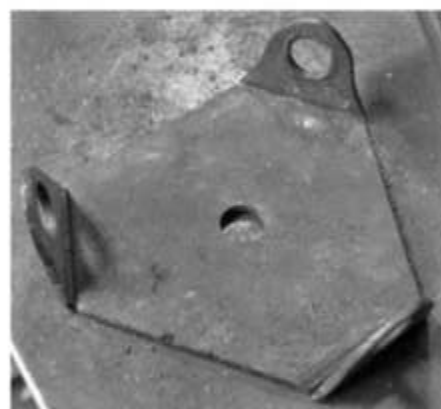
The piece starts as an equilateral triangle. After the holes are punched Stuart rounds the corners with a chisel.
