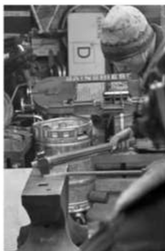
Fullering the feet before bending.
