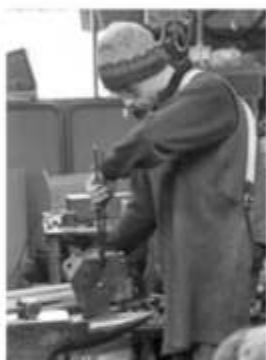
Flattening the bent corners.
