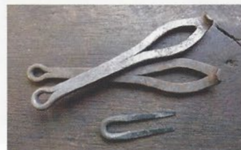
Left: Welded eye hasps and staples. Reproduc- tions. Forged mild steel. Length: 8"
