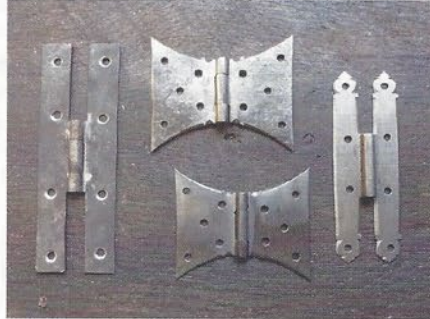
Right: Hinge reproductions. Forged and filed mild steel. Largest hinge length: 7"
