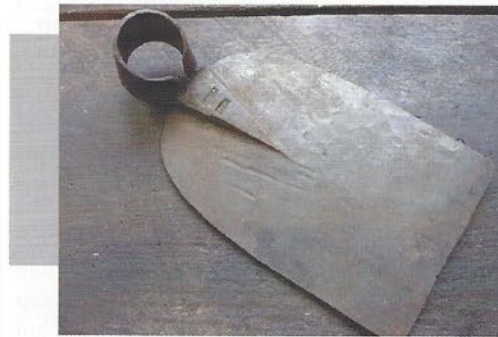
Left: Hoe reproduction. Forged mild steel. Length: 13"
