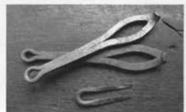
Left: Welded eye hasps and staples. Reproduc- tions. Forged mild steel. Length: 8"
