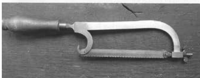
Below: Hacksaw reproduction. Forged filed and turned. Mild steel and beech. Length: 12"
