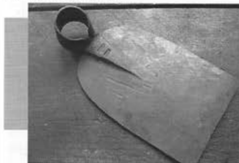
Left: Hoe reproduction. Forged mild steel. Length: 13"
