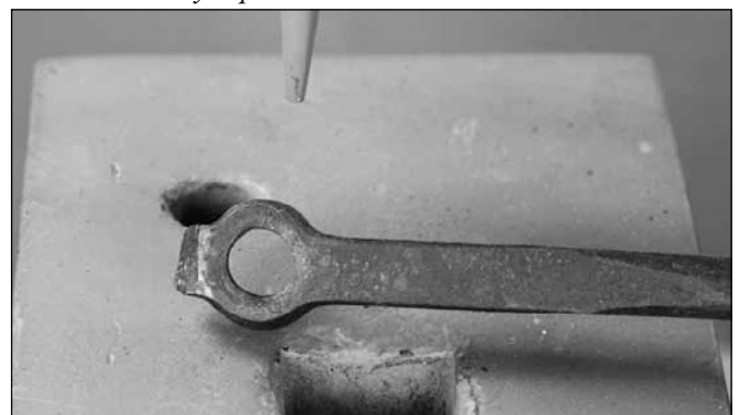
Hot rasp the cut end after drifting to round
