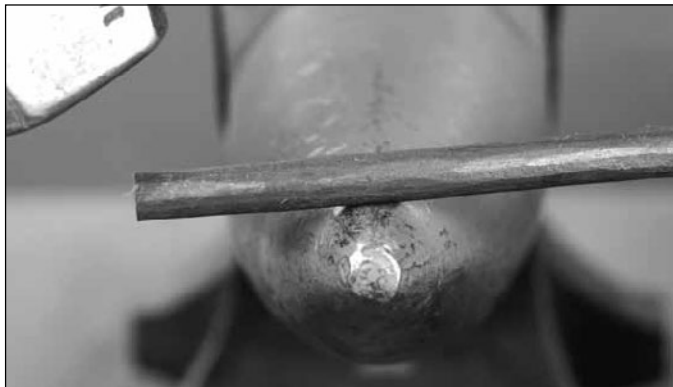
Lay off about 1⅜-inch from the center of the bick
