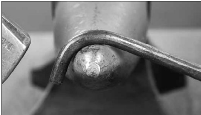
Bending the bar to slightly past 90° makes it easier to thread into the mortise
