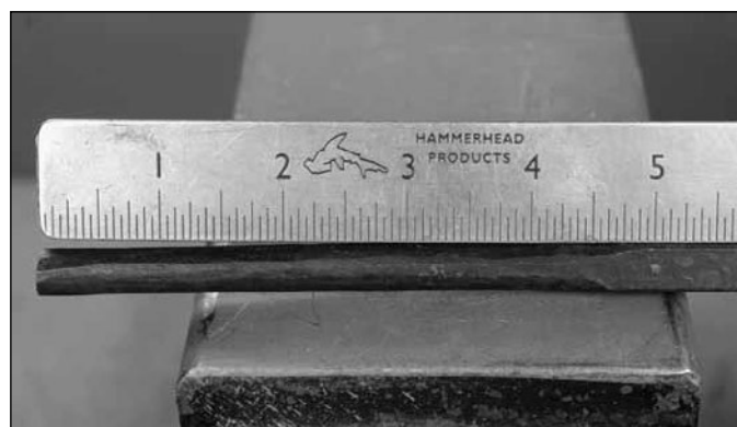
Aim for a 4\frac{1}{2} to 5-inch length of \frac{3}{8} -inch round bar when finished
