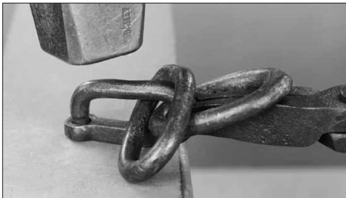
Here is the repair link applied
