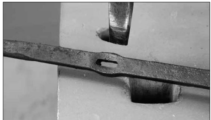
My slot punch is slightly over 3/8-inch wide
