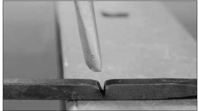
Sever the piece from the bar 1¾-inch past the transition area. Note that I am holding the chisel at an angle to the bar
