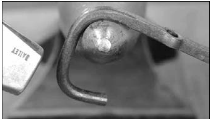
Take the bend past 90° if you can, making it easier to catch the bick when you turn the link over
