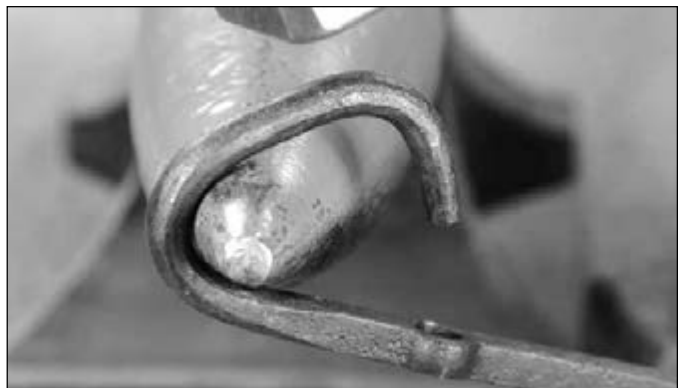
This is as far as I go on the bick before moving to the face of the anvil
