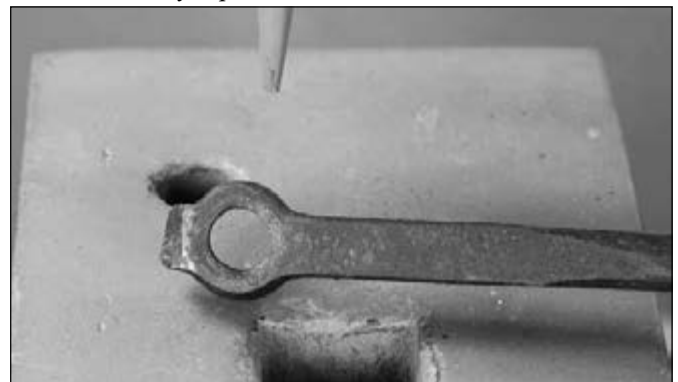
Hot rasp the cut end after drifting to round
