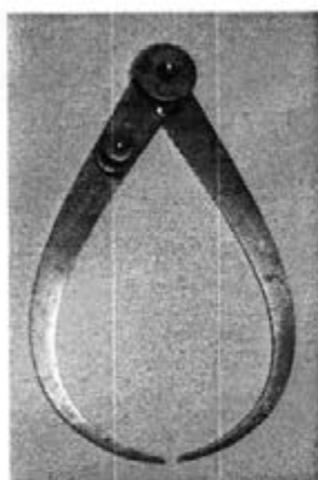
locking outside calipers with fine adjustment
