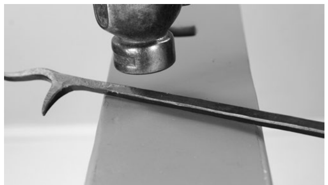
Taper from the poker end to the handle, chamfering the corners as you go.
