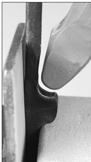
Use a combination of a ½-inch fuller and your cross peen to draw down the pillow of material to a taper
