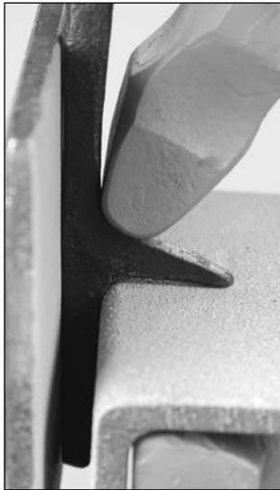
Fuller at the transition area, and cross peen where a mis-hit won't cause indigestion
