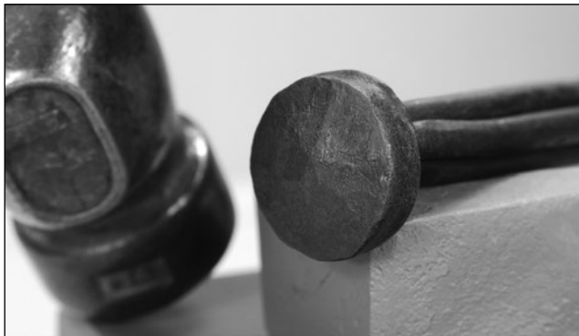
The finished weld, with the collar thinned to 1/4-inch thickness at the edge
