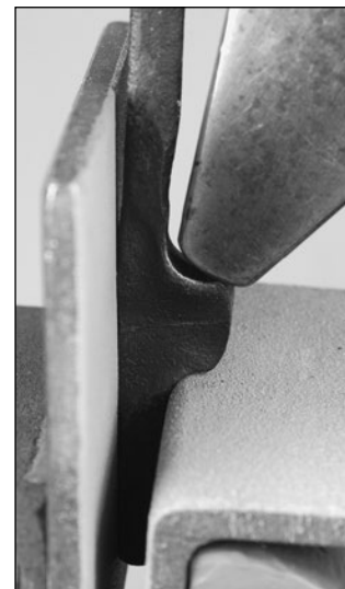
Use a combination of a ½-inch fuller and your cross peen to draw down the pillow of material to a taper
