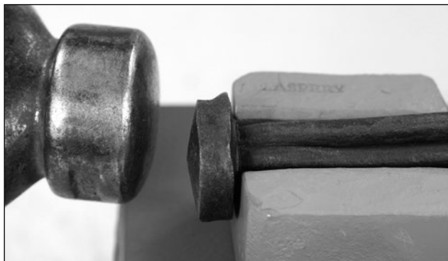
Turn the bar as you work to flatten and weld in the handle material to the collar
