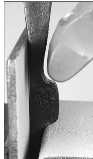
Using a backing plate and jaw insert, clamp the pillow of material up in the vise
