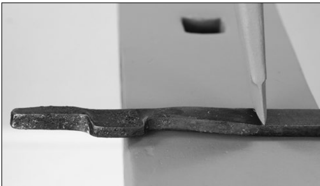
Holding the chisel at an angle away from you, sever the forged end from the parent bar and draw to ¾-inch sq
