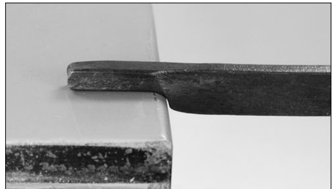
Set the shoulder and draw the material down to 5/16-inch square
