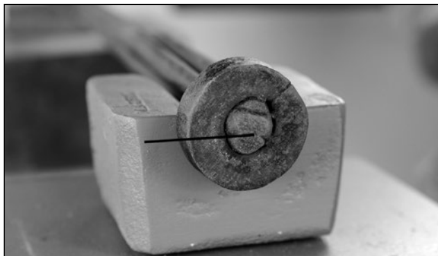
Keep the horizontal centerline of your hammer below the top edge of the swage block
