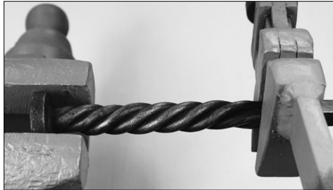
Don't get the twists too tight, or the rods will pop past one another. Twist (for example) clockwise
