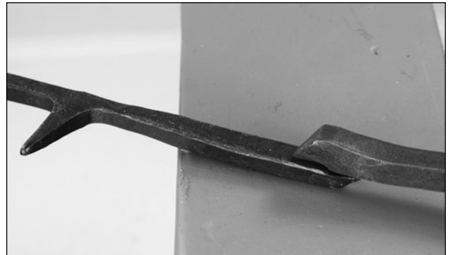
Weld the poker end onto the shaft material and taper the complete shaft aiming for \frac{1}{4} -inch square at the spur
