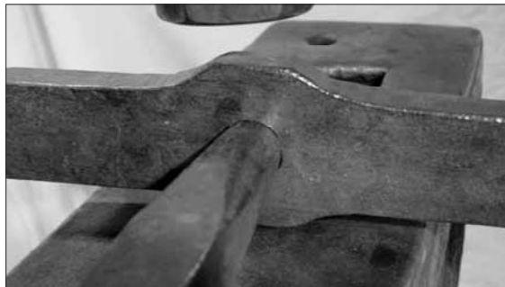
Starting to dress the sides of the blocking. Use light blows so as not to stretch the hole.
