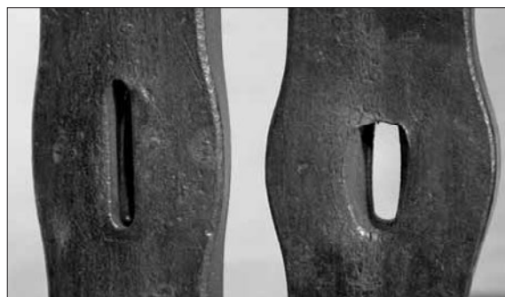
The result of the first upsetting. The original slot on left is shown for comparison.
