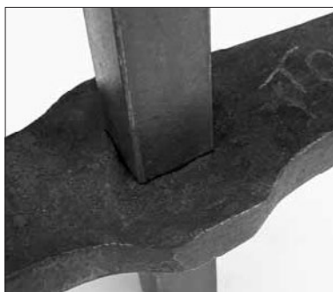
The square blocking complete with a taper to the end of the bar and a tenon drawn.
