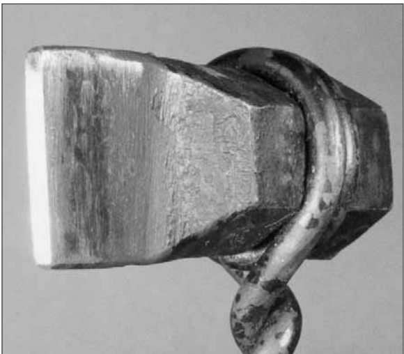
2. Working end of the punch, ⅛" thick and flat.
