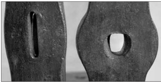
The result of the second upsetting. Note the shape of the hole in the back differs from the front.
