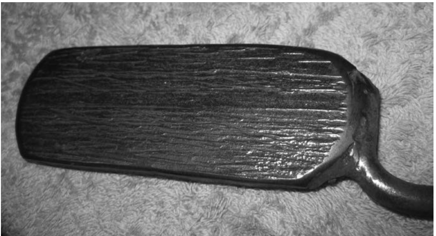
Photo 11: Hand Held Paddle Die Created from Power Hammer Die in Photo 2
