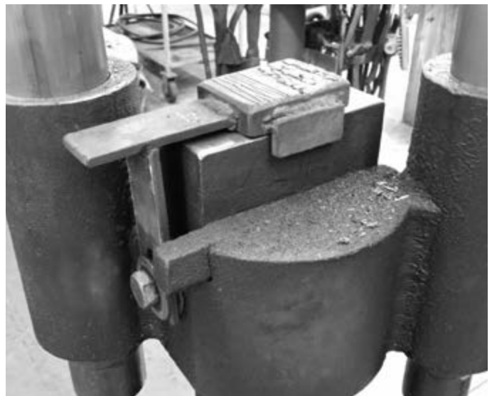
Photo 8: Texture Tool on the KA-75
