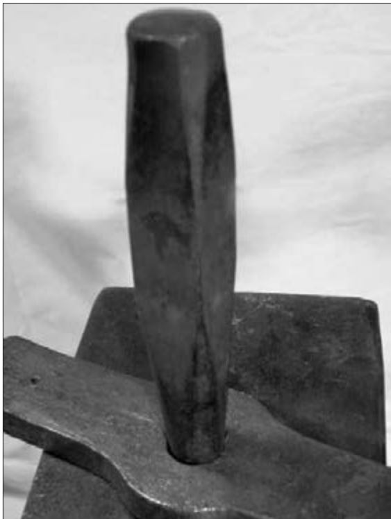
Starting to drift. Note that the sides of the drift are parallel to the sides of the bar.
