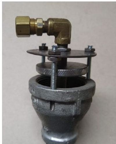
Right: Support bridge can be connected to pipe fitting reducer or custom forged reducer to accommodate the air flow adjusting disc.
