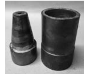
Top: Sch. 40 pipe on left, upset, forged truncated reducer on right. Below: Die set used with a 40 ton hydraulic press.
