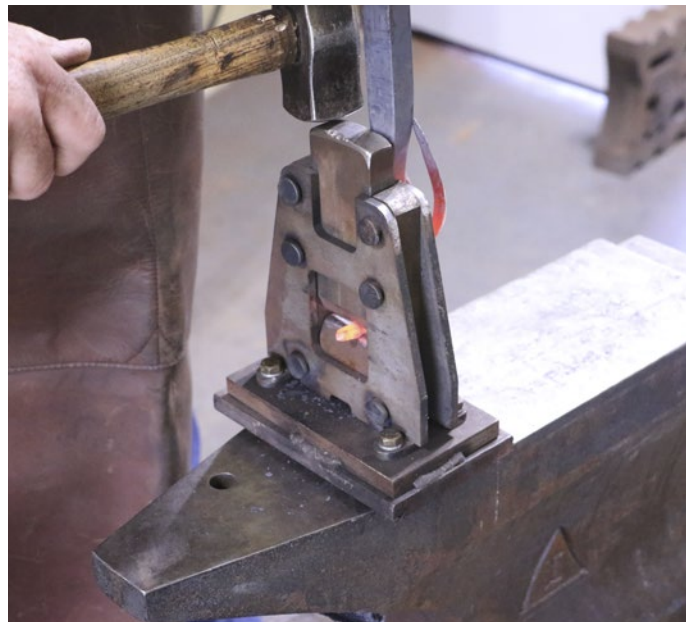
Photo 38: Drawing Out Beard with Smithin Magician
