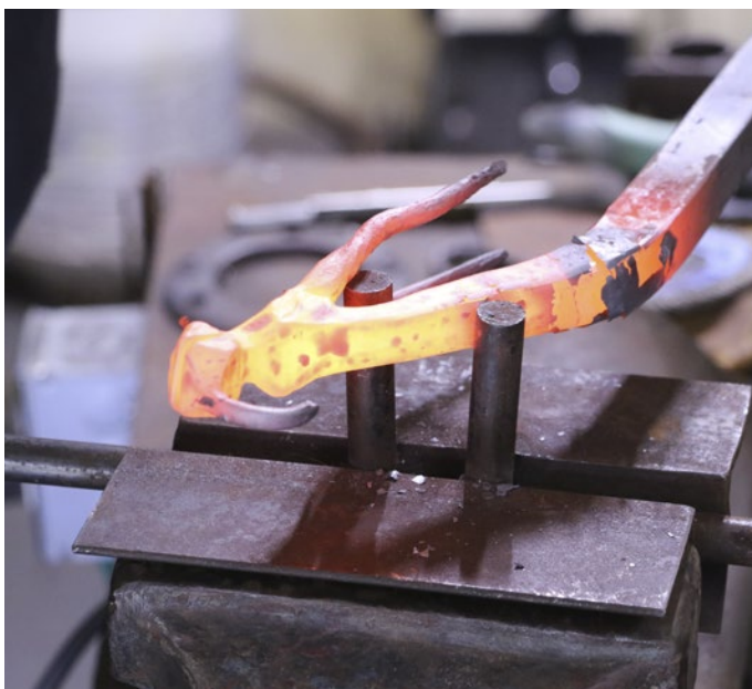
Photo 50: Bending the Neck Forward
