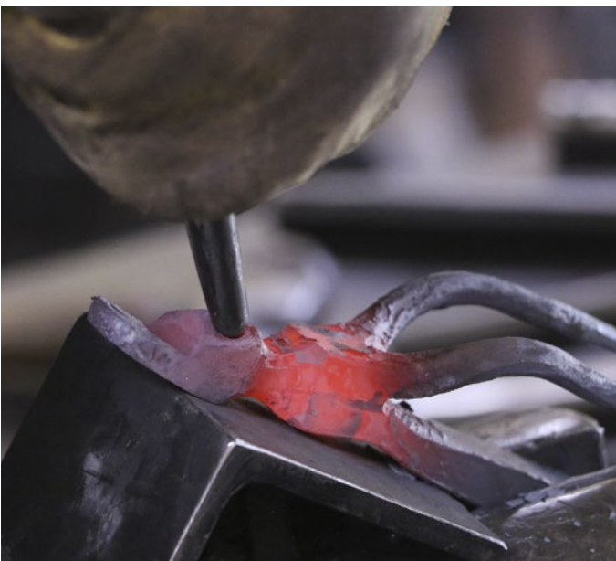
Photo 24: Punching the Nostrils with Center Punch
