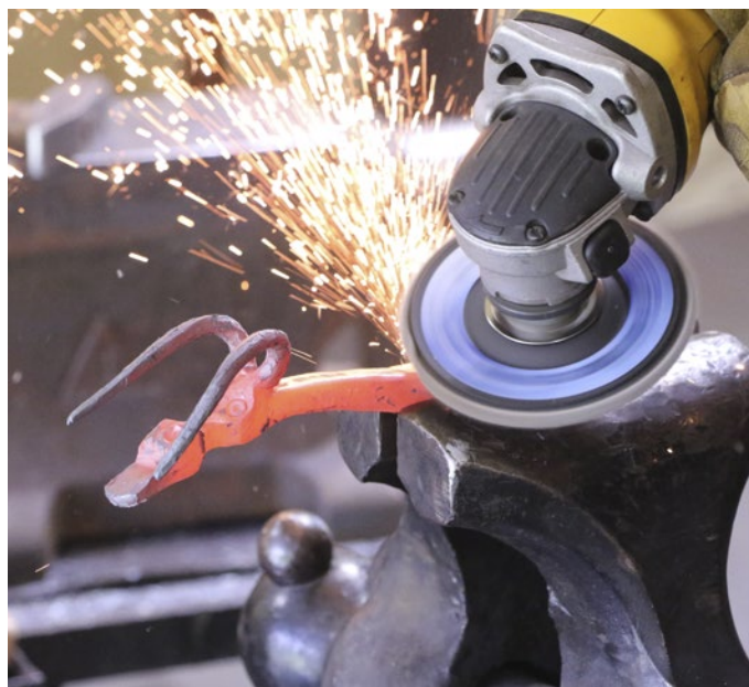
Photo 34: Cleaning the Surface with a Flap Disc
