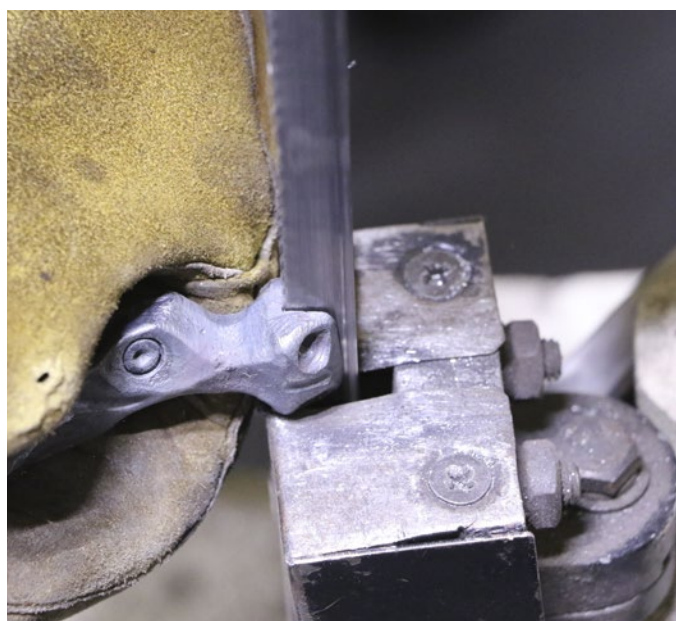
Photo 42: Sawing the Mouth
