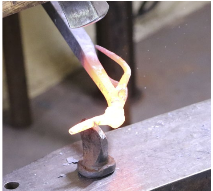
Photo 37: Cutting Off Excess Beard Material
