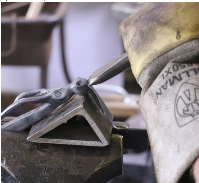
Photo 40: Marking the Mouth Line with a Chisel
