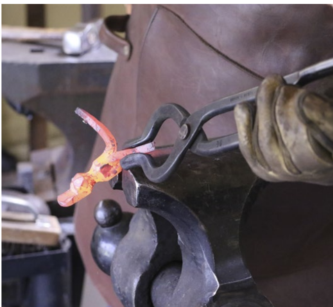
Photo 20: Convenience Bends for Rounding the Horns
