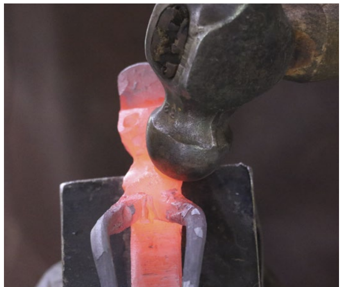
Photo 26: Depressing the Eye Sockets
