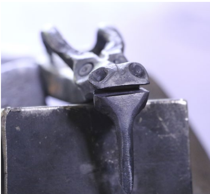
Photo 45: The Mouth After Bending Open
