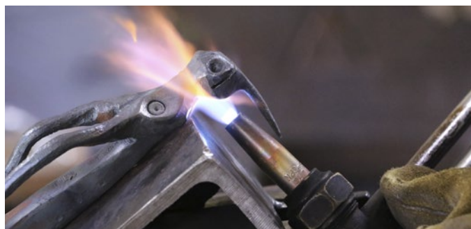
Photo 43: Heating the Mouth Prior to Bending Open
