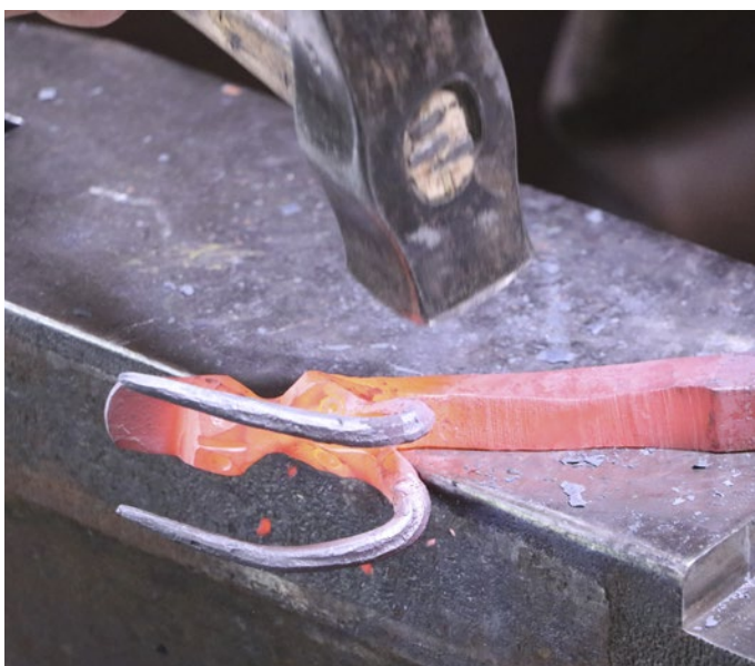
Photo 32: Hammering the Neck
