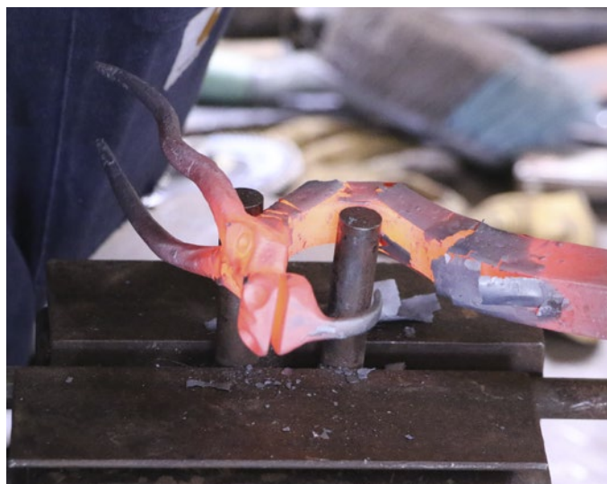
Photo 51: Finishing the Forward Bend
