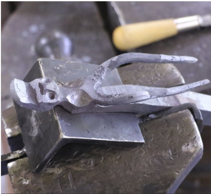
Photo 27: The Progress After Dishing the Eye Sockets
