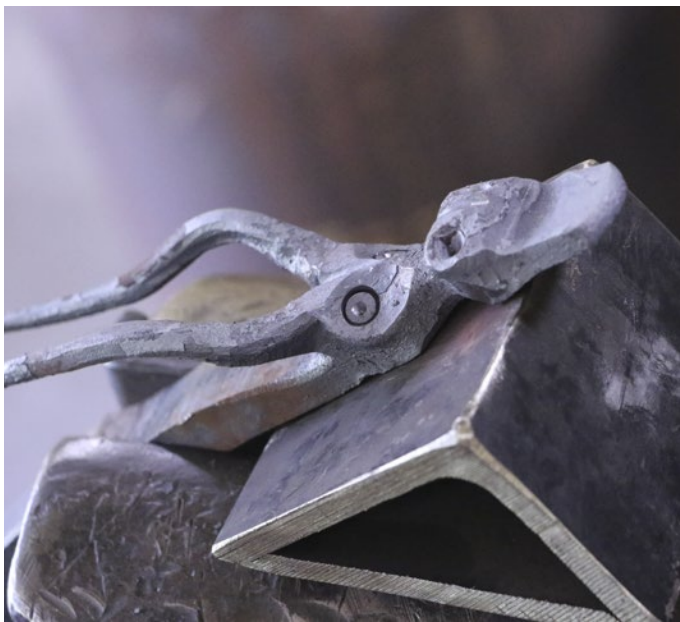
Photo 31: Progress After Punching the Eyes
