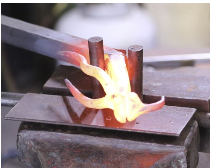
Photo 49: Bend the Base of the Neck Backward
