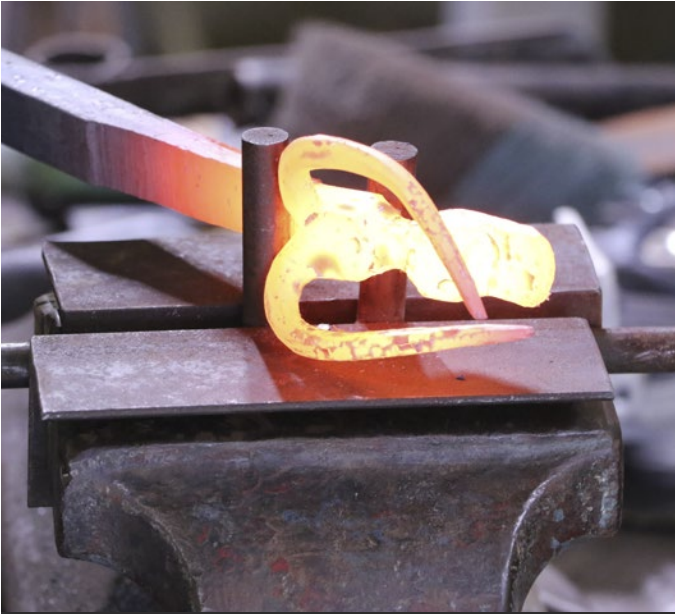
Photo 23: Keeping the Head in Line Using Adjustable Bending Forks
