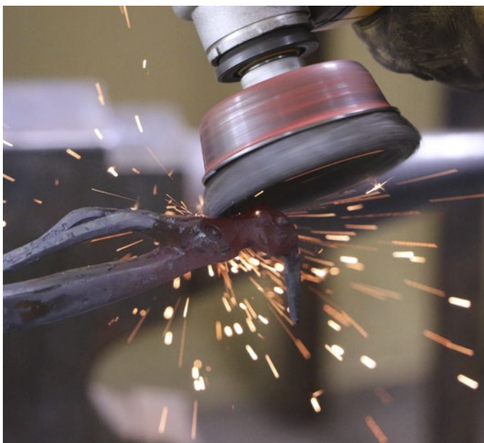
Photo 39: Hot Brushing with Wire Cup Wheel
