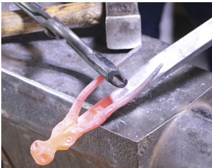
Photo 48: Bend the Horns Up to Gain Clearance
