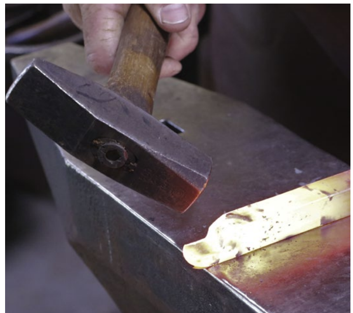
Photo 3: Making the Flats for the Nostrils
