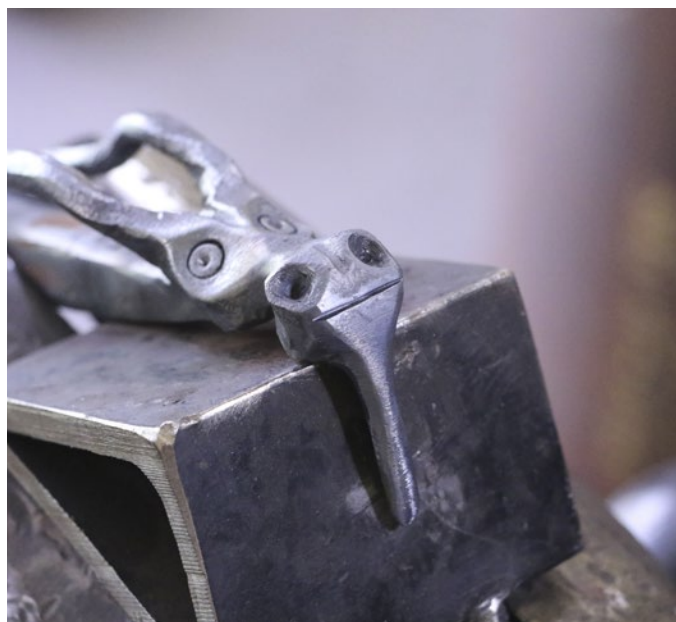
Photo 41: Mouth Marked and Ready for Sawing
