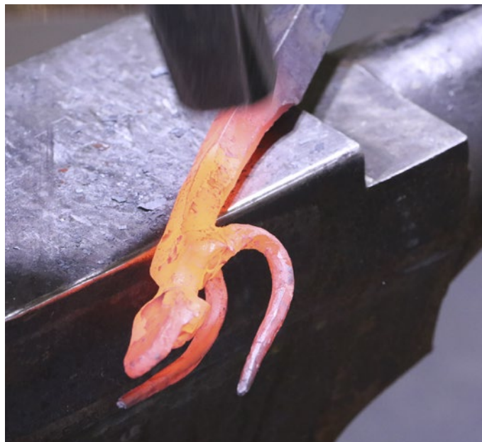
Photo 33: Softening the Corners of the Neck
