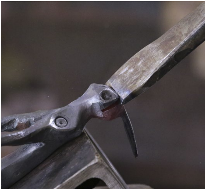
Photo 44: Opening the Mouth with a Chisel
