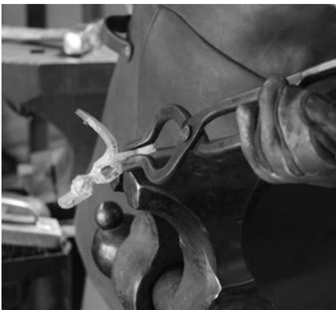
Photo 20: Convenience Bends for Rounding the Horns
