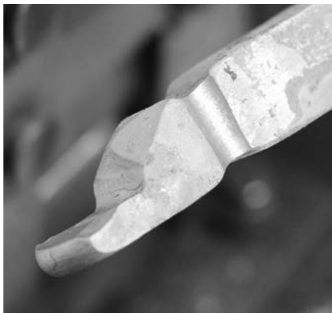
Photo 6: Fullered on Top and Sides of Cheek Area hammer now if you need to.
