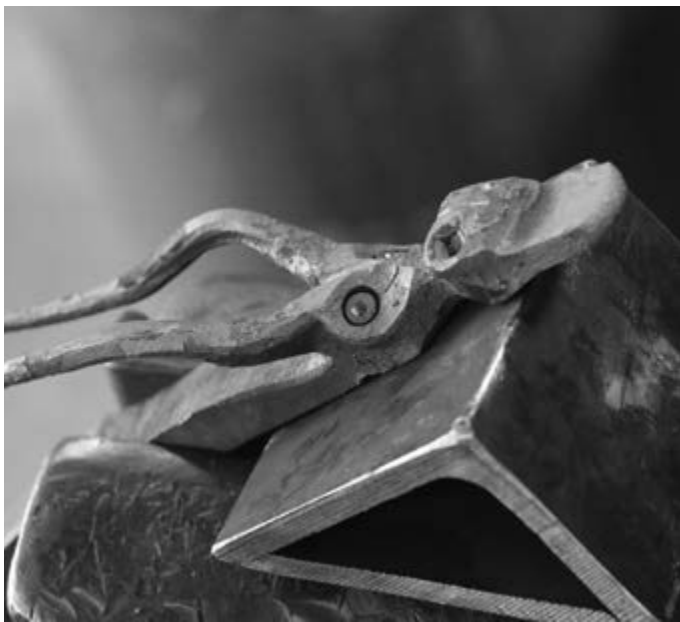
Photo 31: Progress After Punching the Eyes
