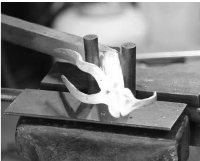
Photo 49: Bend the Base of the Neck Backward
