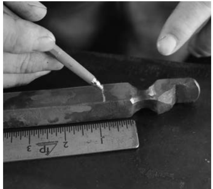
Photo 10: Reference Line for Base of Horns
