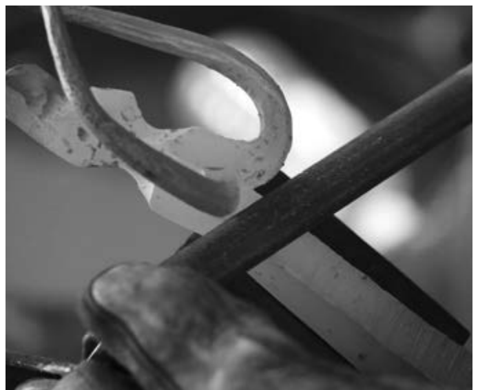
Photo 22: Hot Filing to Clean Up the Rounded Horns
