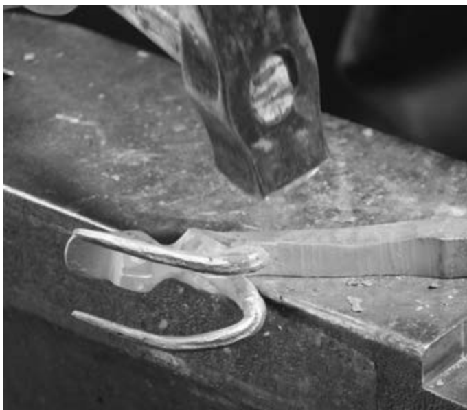
Photo 32: Hammering the Neck
