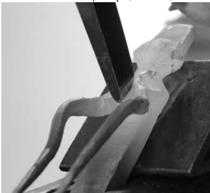
Photo 28: Fullering Between Eye Sockets
