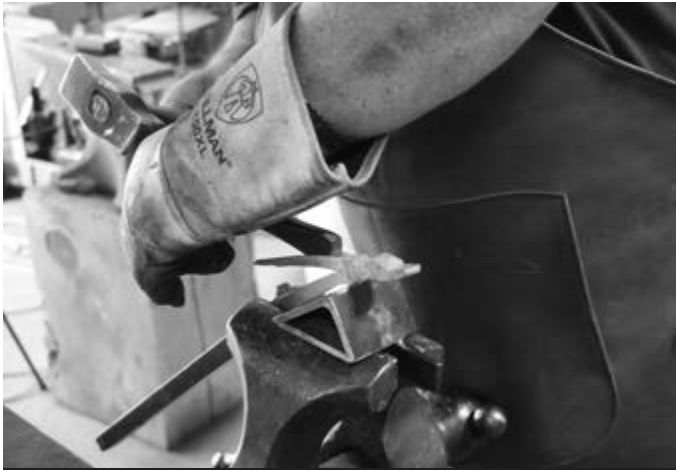
Photo 18: Cleaning Up the Horn Base Cuts with Chisels and Files
