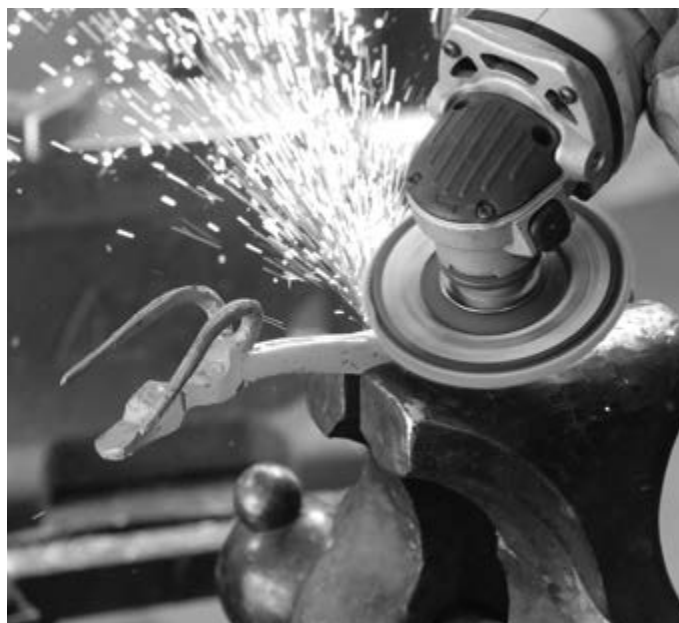
Photo 34: Cleaning the Surface with a Flap Disc
