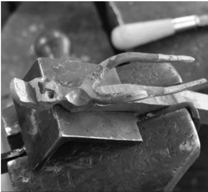
Photo 27: The Progress After Dishing the Eye Sockets
