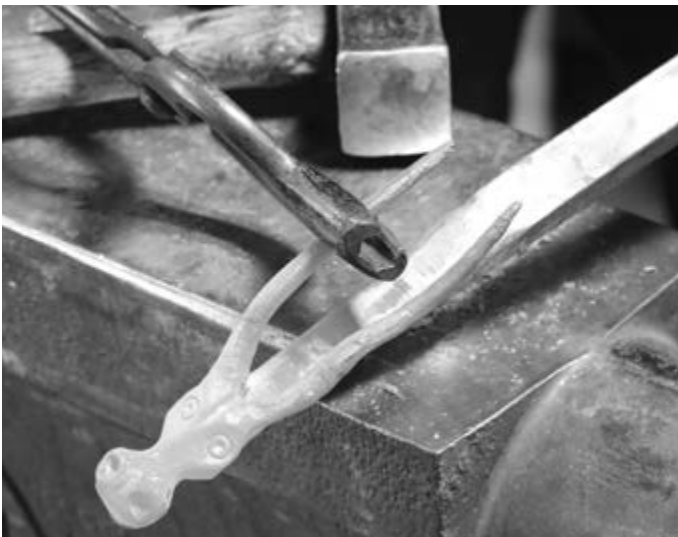
Photo 48: Bend the Horns Up to Gain Clearance
