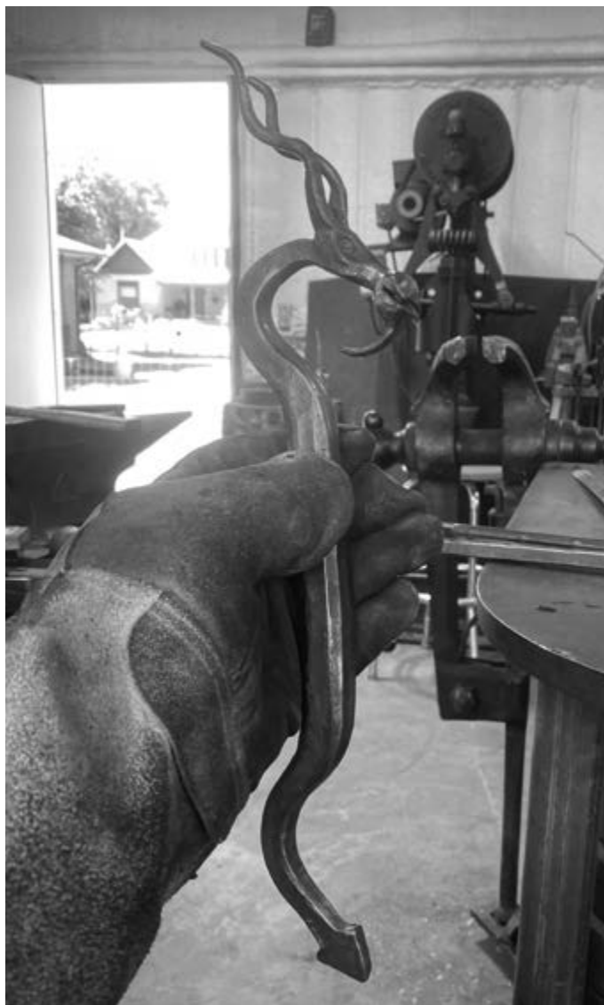
Photo 52: A Dragon Head Door Pull Ready for Attaching to the Backing Plate
