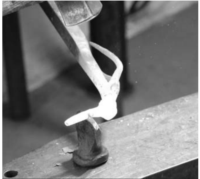
Photo 37: Cutting Off Excess Beard Material
