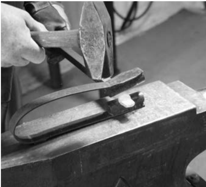
Photo 8: Enlarging the Cheek Fullering
