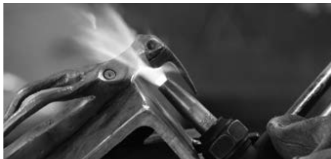
Photo 43: Heating the Mouth Prior to Bending Open
