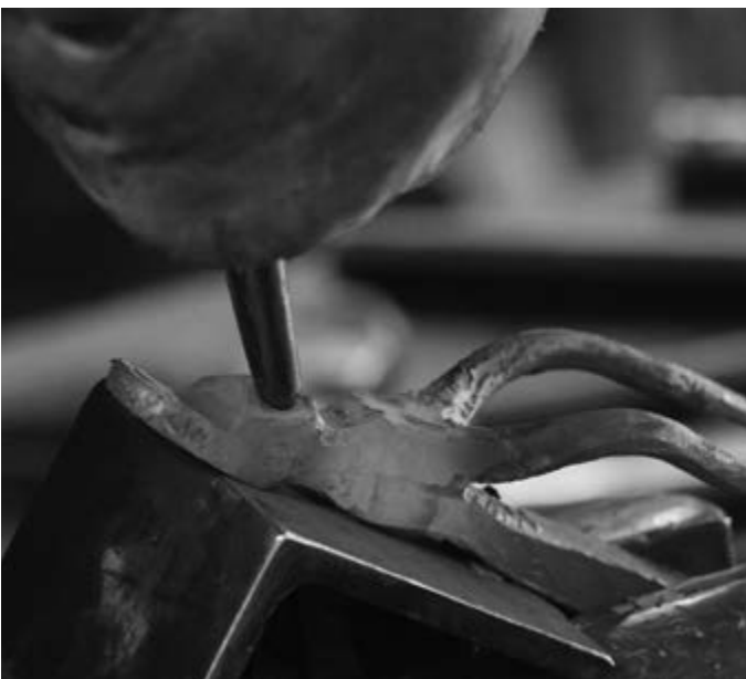
Photo 24: Punching the Nostrils with Center Punch
