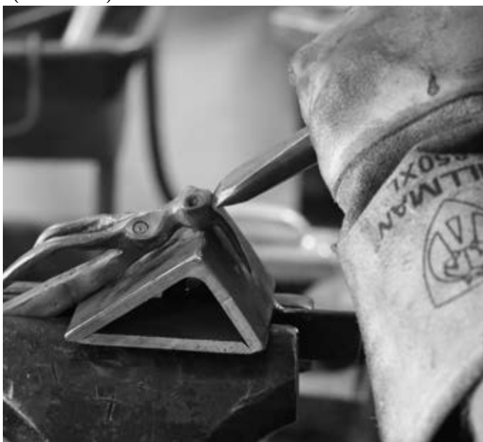
Photo 40: Marking the Mouth Line with a Chisel
