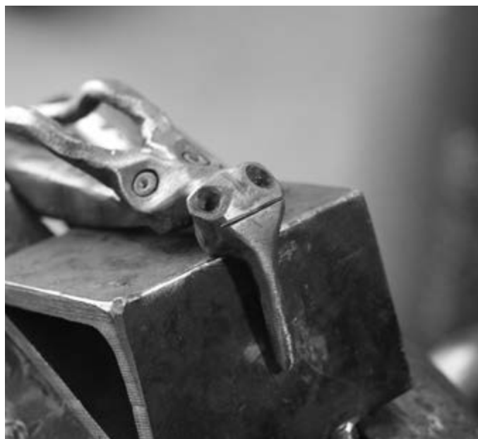
Photo 41: Mouth Marked and Ready for Sawing
