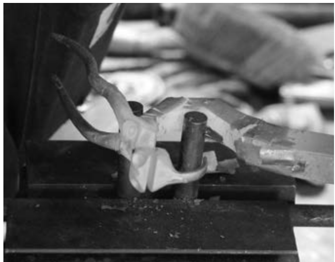
Photo 51: Finishing the Forward Bend
