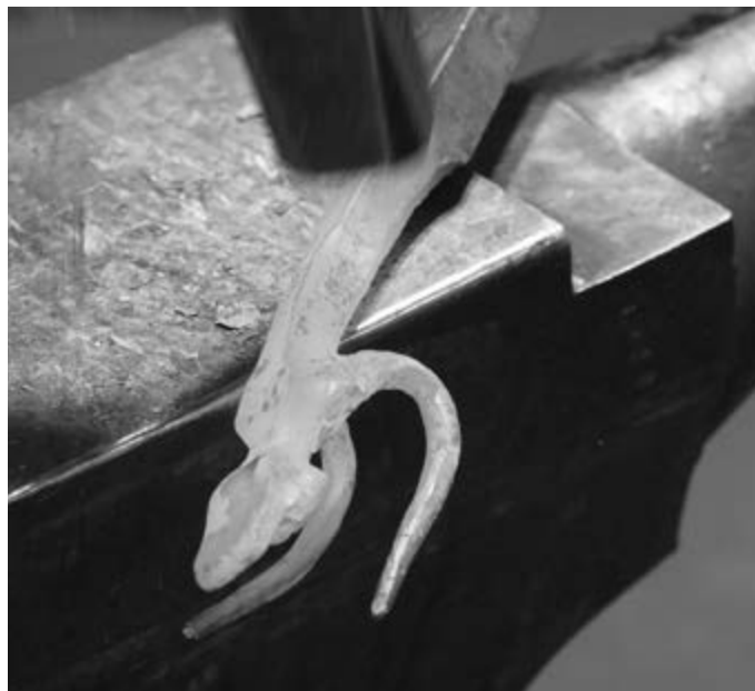
Photo 33: Softening the Corners of the Neck
