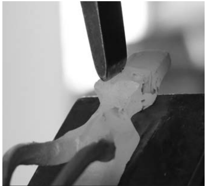
Photo 29: Fullering Between Nostrils
