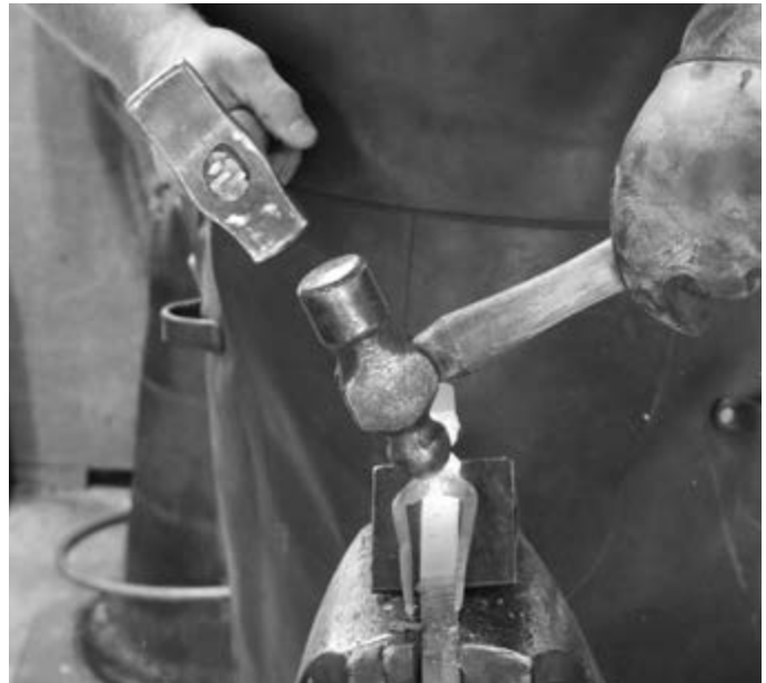
Photo 25: Depressing the Eye Sockets (Use a Soft Hammer to Strike!)
