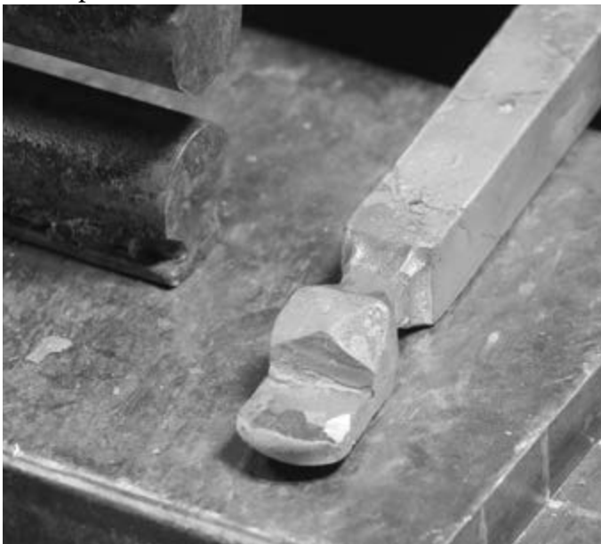
Photo 9: Progress After Fullering
