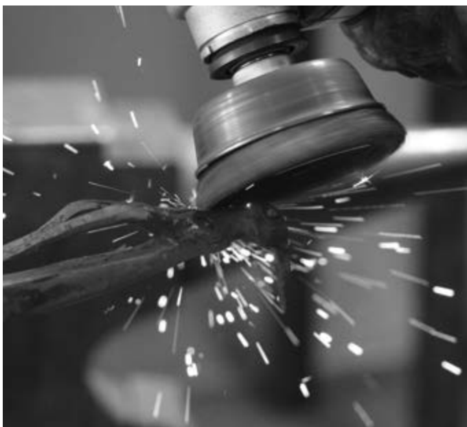
Photo 39: Hot Brushing with Wire Cup Wheel
