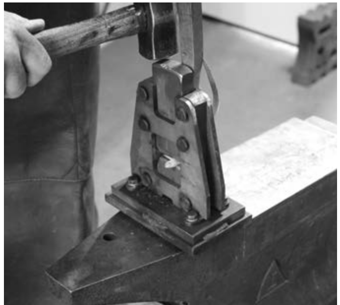
Photo 38: Drawing Out Beard with Smithin Magician
