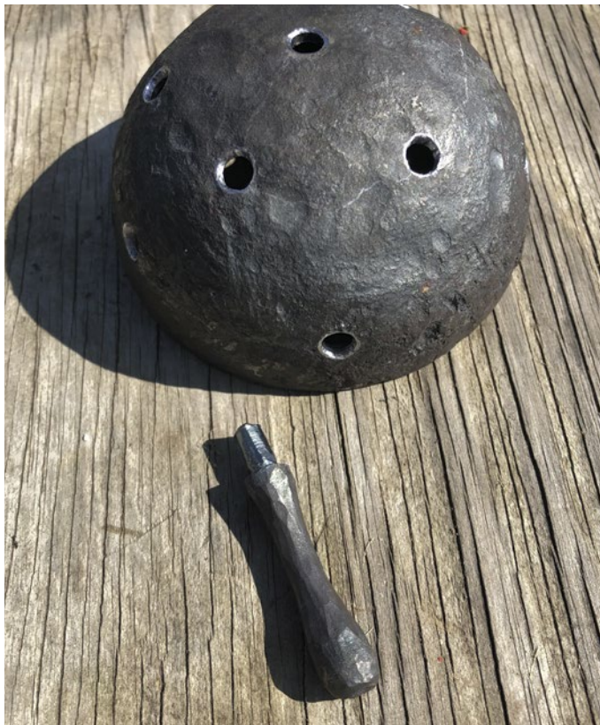
Holes Drilled and Ready for the Spikes
