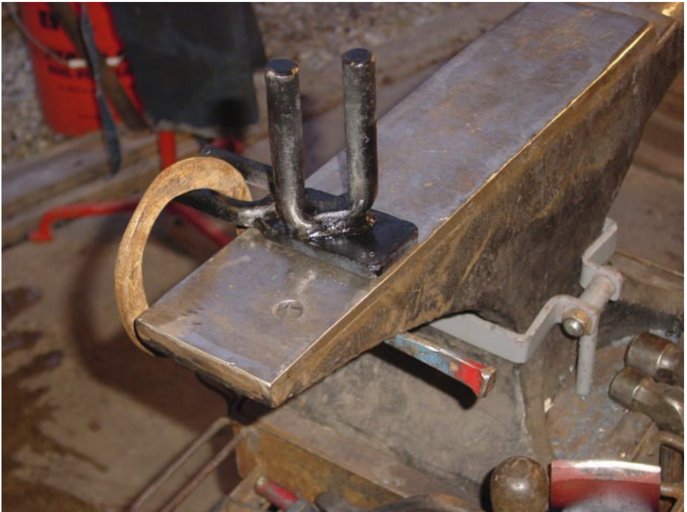
Photo 02: The Multi-Fork Secured in the Hardie Hole with Tapered Pin
