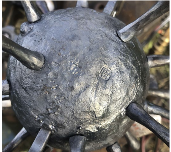
The Weld After Peining (To Hide It)
