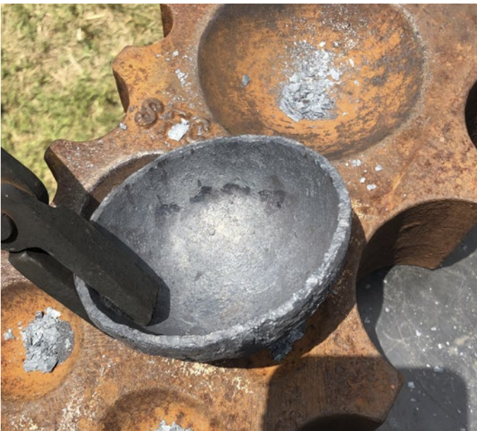
Second Pass of Dishing with Heat
