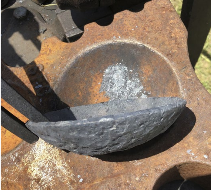
First Pass of Dishing with Heat
