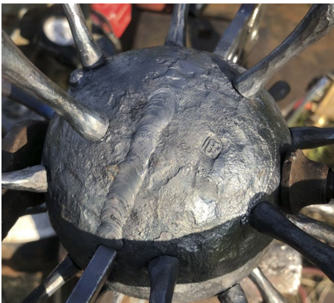
The Two Halves Welded Together
