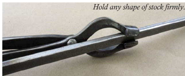
Works well as bolt tongs.
