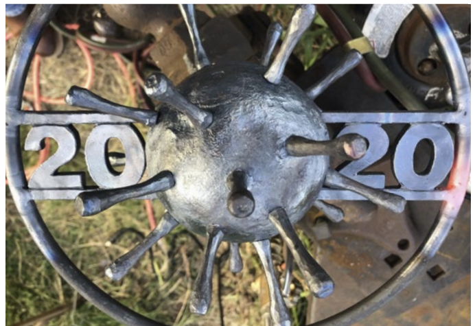
The Support Bar Torch Welded to the Gate Ring
