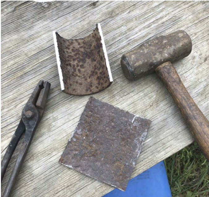
Flattening the Pipe Halves to Make Material for Dishing
