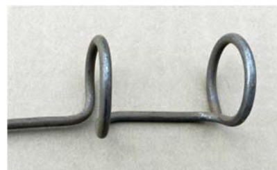
Put a 90 degree bend in the second hoop.
