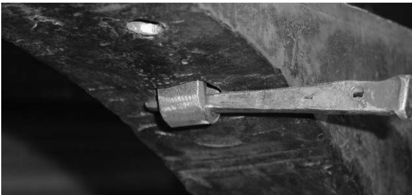
Photo 04: The Hardie Stem with Tapered Pin in Place
