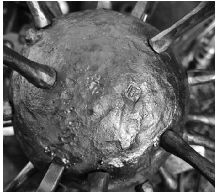
The Weld After Peining (To Hide It)
