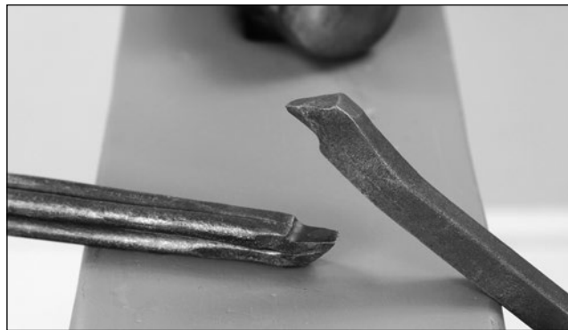
Roll the handle material (that's in your hammer hand) onto the face of the anvil
