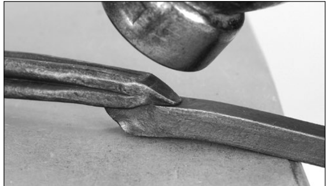
Use the heel of your hammer to weld in the scarf of the handle material
