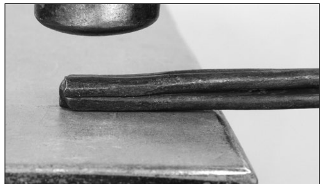
Quickly turn the stack so that two bars are resting on the anvil and forge the bar into a square cross section
