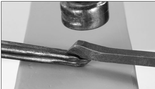
Deliver your first blow to the top of the weld area
