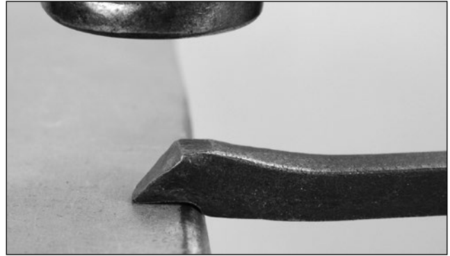
Create the step to the scarf and refine the slope to the toe
