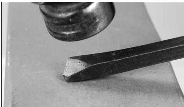
Lift the bar slightly and thin the toe of the scarf, keeping the toe centered on the bar
