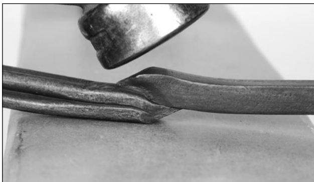
Your next 2 or 3 blows are to weld in the scarf to the handle material
