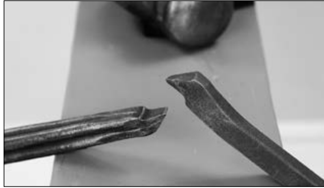
Touch both bars to the sides of the anvil
