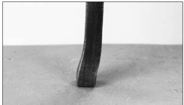
Nothing good ever follows continuing to forge a bent or twisted bar! Take the time to straighten the upset end
