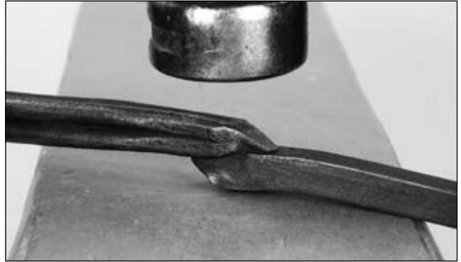
Turn the stack over and give a blow to the top of the weld area
