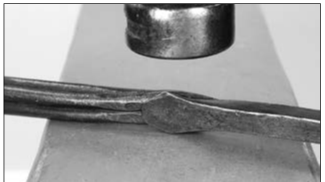
Work the sides and corners of the weld only after you are sure that the weld is good
