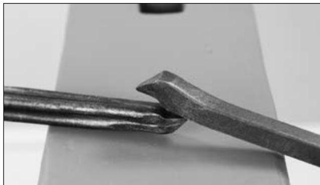
Roll the handle material (that's in your usual tong hand) down to trap the handle
