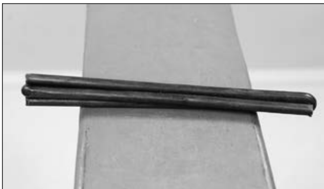
The ends should all be equal. If one end is better than another, weld the better end first
