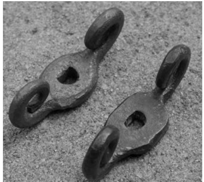
Upper left is punched and drifted (better result.) Bottom right is drilled and drifted but requires cleanup with the hammer.
