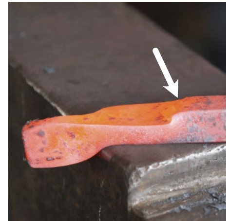
Use half-faced blows here. Dig in to the parent bar with the heel of the hammer
