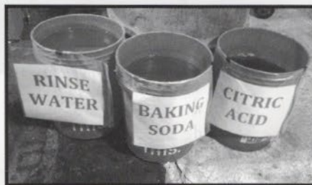
Acid bath and neutralizer speeds a shiny finish, ready for final coatings.
