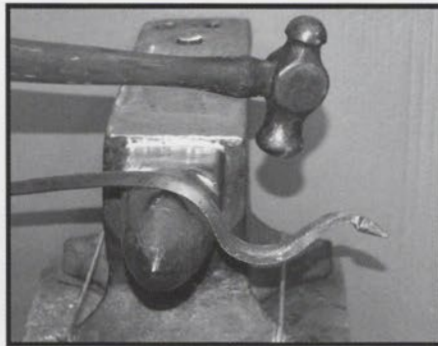
Curving the snake body over the anvil's horn, using the round-faced hammer.
