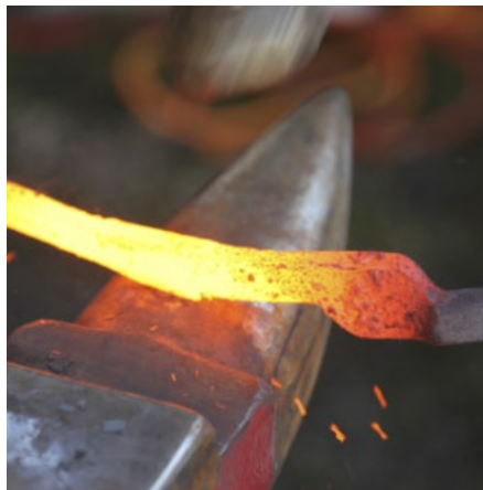
Draw down the reins over the bick for efficiency and dress on the anvil face
