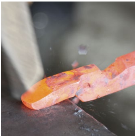
The end is drawn to a slight taper
