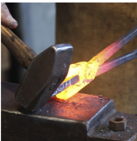
Adjust the jaws of the tongs by using the appropriate sized stock and closing the jaws
