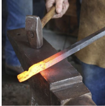
Again, turn the top of the bar away from your hammer hand
