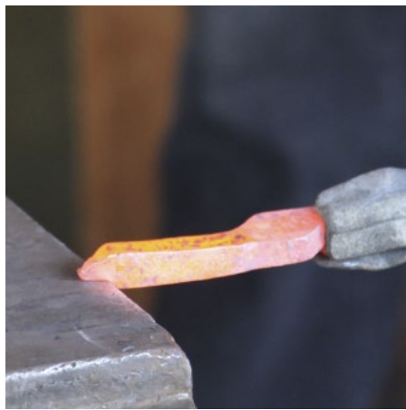
Create the step of the weld scarf
