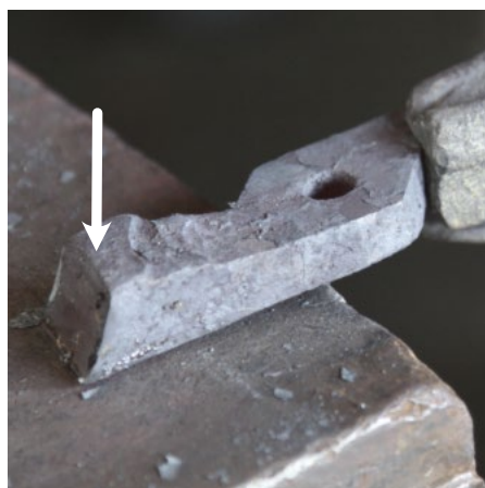
Also preserve the slope of the cut to help with the weld scarf as you work
