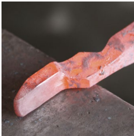
The taper helps the tongs slip past coals in the fire and pick up stock
