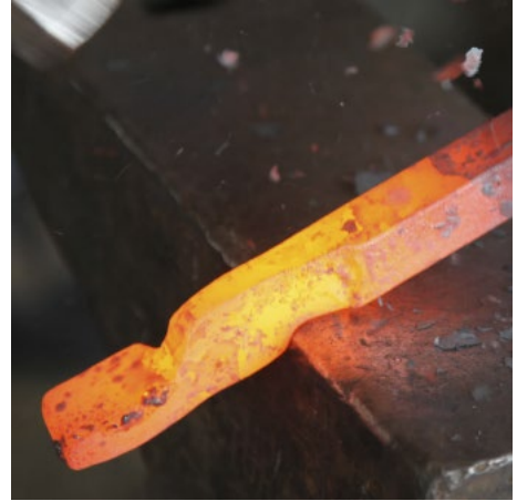
Use half-faced blows to define the rear of the boss
