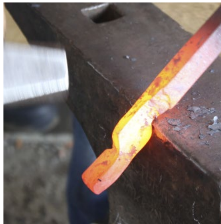
Dress the front of the boss over the offside edge of the anvil
