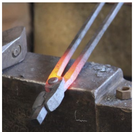
Once adjusted, quench the jaws and adjust the reins to suit your grip
