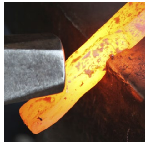
Mark likes a parallelogram-shaped boss to prevent the reins from swinging open
