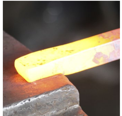
Walk the hammer towards the end of the bar
