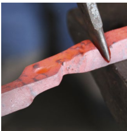
Sever the jaw and boss assembly from the parent bar
