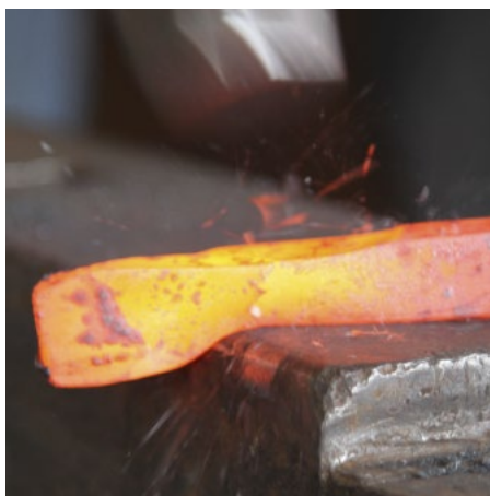
Hold bar at an angle to the offside edge and draw down the boss
