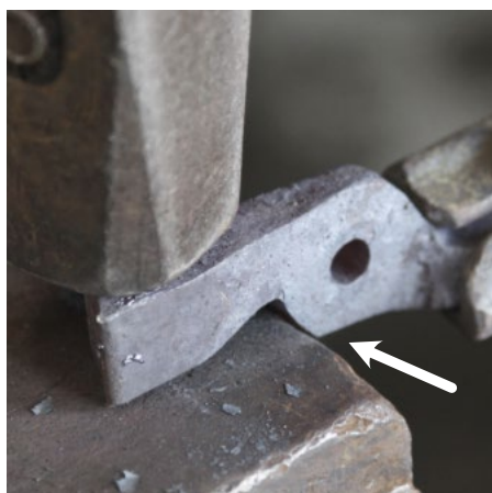
Protect the corner of the boss as you draw down the rein
