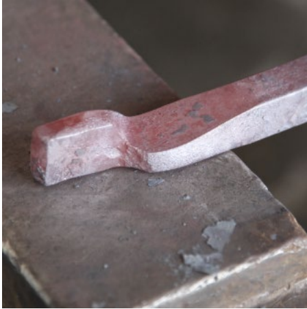
The boss is half the parent bar thickness for at least the width of your hammer
