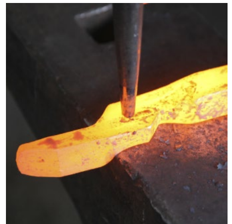
Place the jaw over the offside edge to begin your punched hole
