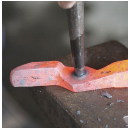
Drift to rivet size over the pritchel hole
