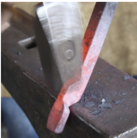
Work equally from all sides of the boss
