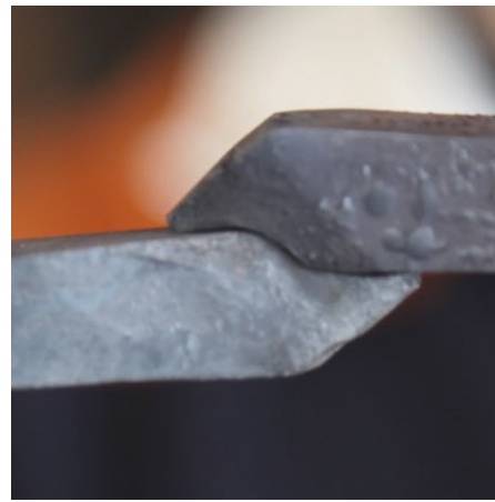
One of the secrets to forge welding is to make sure the scarfs fit before welding
