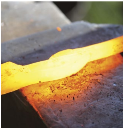
Make the weld, ensuring that the toe of both scarfs are blended into the other stock
