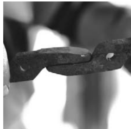
If you are consistent in your work the jaws should fit together without modification
