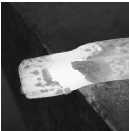
Draw to \frac{1}{2} -bar thickness. Turn the top of the bar away from your hammer hand
