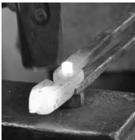
Round bar will serve as a rivet, with a spacer (nut) to help with even distribution
