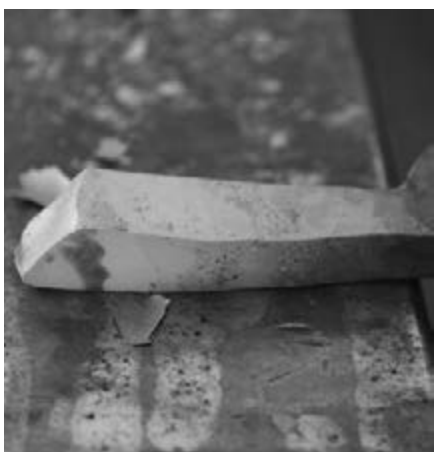
Working from just two sides helps preserve the slope and makes an easy scarf prep
