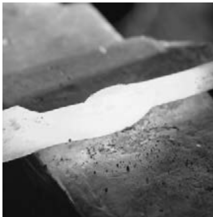
Make the weld, ensuring that the toe of both scarfs are blended into the other stock
