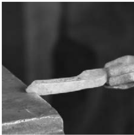
Create the step of the weld scarf
