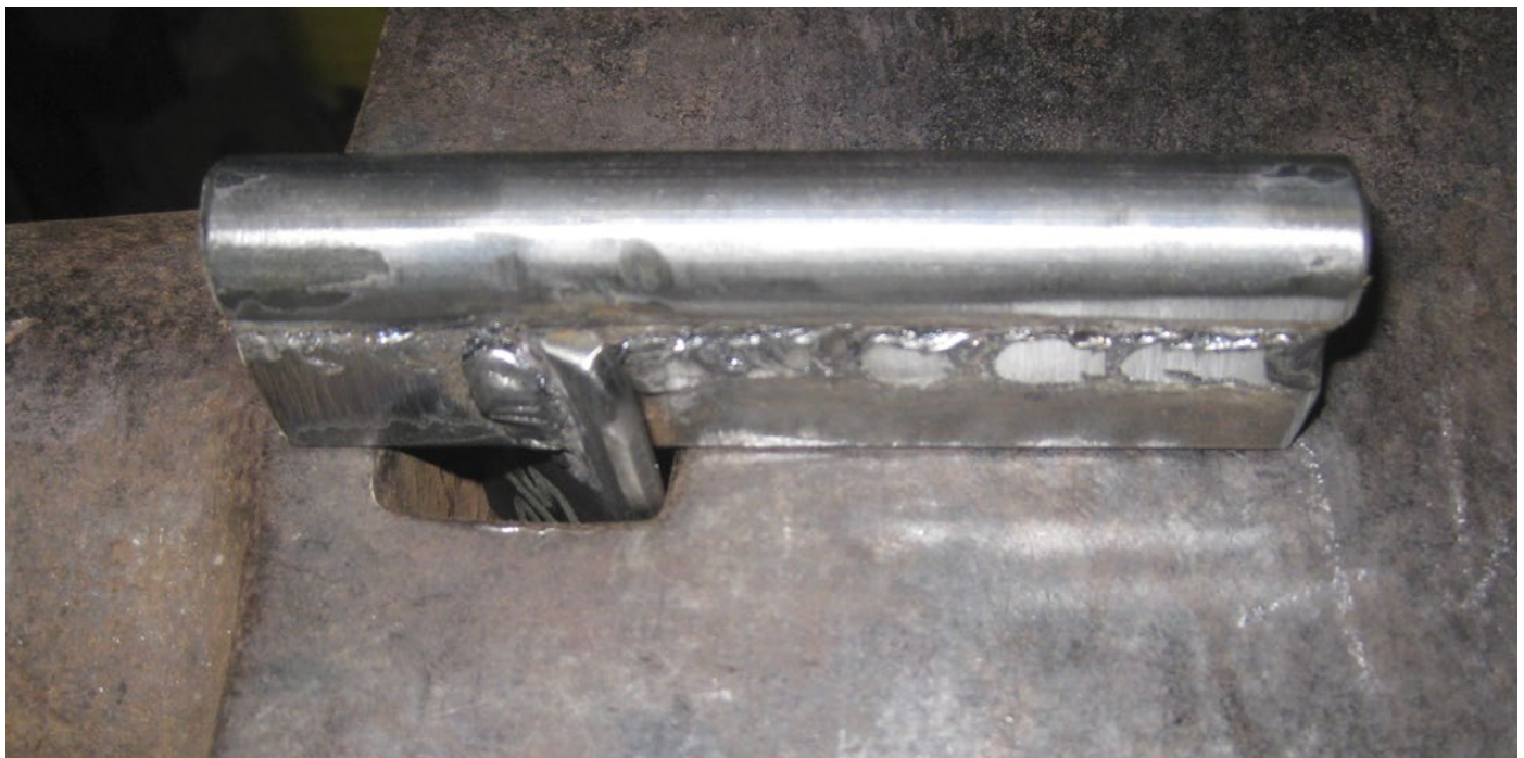
Photo 5: \frac{3}{4} " fuller on the anvil ready to work
