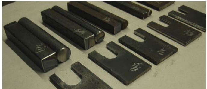
Photo 3: Parts ready to weld. Square bar on bottom, round bar on top. (Notice I slipped in a set of \frac{5}{8} " material)
