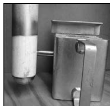
Above photo shows how the PVC pipe, attached ball and 5/8" pin sit inside forge for casting step.
