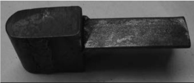
Photo 1: 1" fuller made by Mark Aspery about ten years ago inspired this set of bottom fullers
