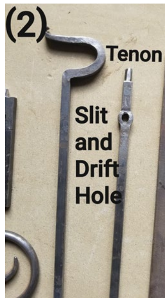
Swing bar with a "Slit and Drift" hole and tenon. See Mark Aspery "Mastering The Fundamentals Of Traditional Joinery". Excellent book.
