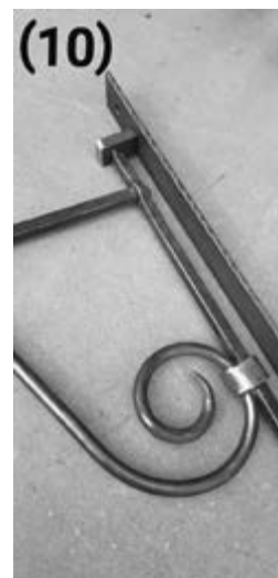
Slip the swinging assembly into the top tenon bracket.
