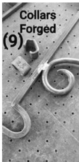
Collars forged and ready to be applied
