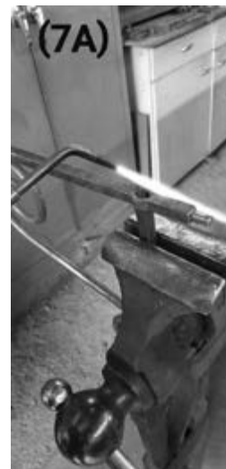
Heating and forging the tenon head
