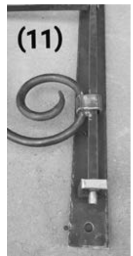
Slip the swinging assembly into the bottom tenon bracket and weld that bracket to the mounting bar.
